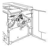
2 Grasp the release lever on the OPC drum cartridge, and then pull the cartridge straight out about 6 inches (152 mm).
