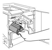
4 Support the middle of the cartridge with your left hand, and then pull out the cartridge.
