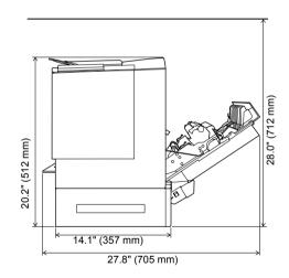
If you have added the optional lower feeder unit, the printer's height will increase by approximately 5" (125.5 mm).
