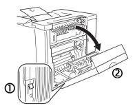
If you have lower feeder unit attached, you first need to open the lower right-side door.
