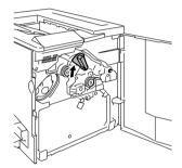
2 Grasp the release lever for the OPC drum cartridge, and then pull the cartridge straight out about 6 inches (152 mm).
