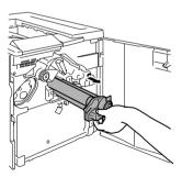
3 Support the bottom of the drum with your hand, then carefully pull the cartridge toward you and remove it.
