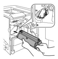
The printer must complete a 150-second calibration cycle after any consumable has been replaced. If you open the door before the message window reads IDLE/MAGICOLOR 2300DL, the printer stops and repeats the calibration cycle.
