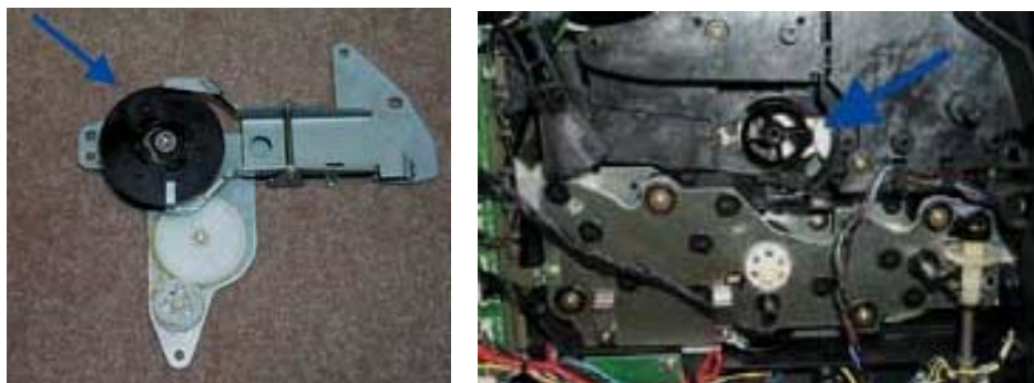
Figure 2a & 2b. The black wheel is spring-loaded and engages and disengages with the hub on the toner cartridge.
