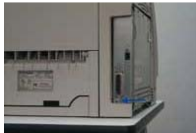
Figure 7b. The fourth controller board screw is located in the back left-hand corner under the parallel port.
