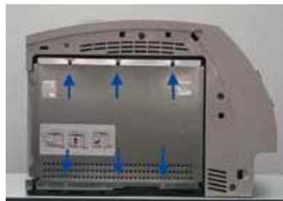
Figure 6. Next, loosen the six outer controller board screws and remove the metal shield.
