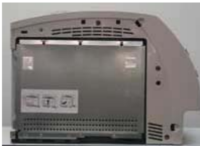
Figure 1. The developer drive is located on the left side behind the printer's controller board.
