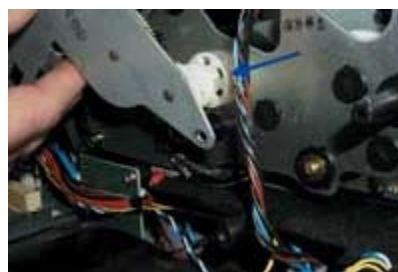
Figure 9. When installing the new developer drive assembly, make certain the plastic wheel is aligned with the hub on the main drive assembly.
