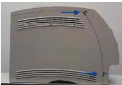
Figure 5. To replace the developer drive assembly, first remove the left panel by releasing the latches.
