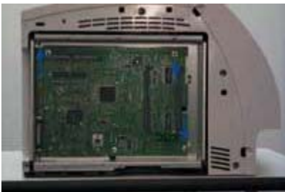
Figure 7a. To remove the controller board, remove two screws on the right and one in the upper left-hand corner.
