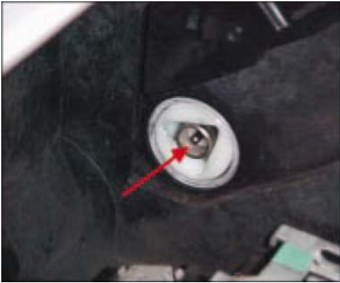
Figure 4 - Toner sensing pin (red arrow).
