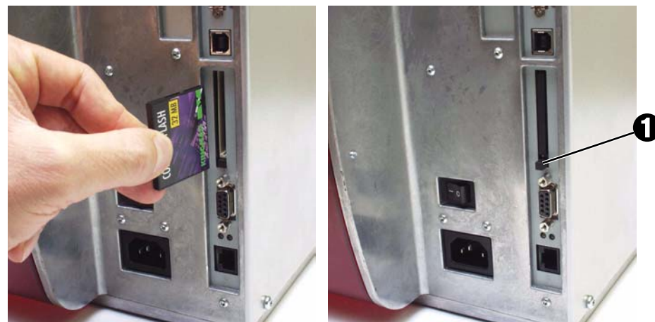
Fig. 12: Inserting a Compact Flash card into a 9854 printer. If the Compact Flash card is inserted correctly, it sits flush with the printer's back wall (right).
