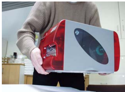
Fig. 2: When lifting the printer, grip under the baseplate!
