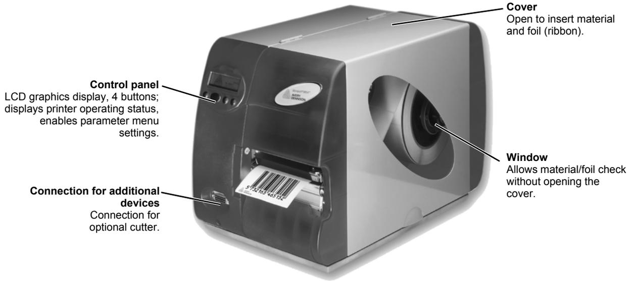
Fig. 4: Exterior view of the printer.
