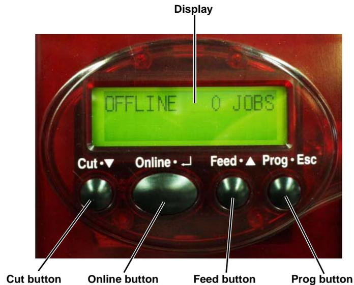
Fig. 14: Control panel for the AP 5.4.
