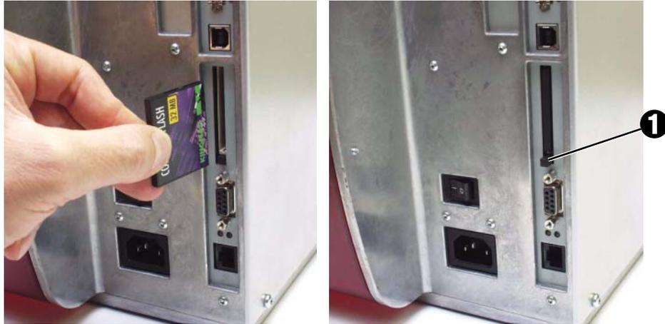
Fig. 17: Inserting a CF card. If the CF card has been inserted correctly, then it will sit flush with the printer's back casing (right).
