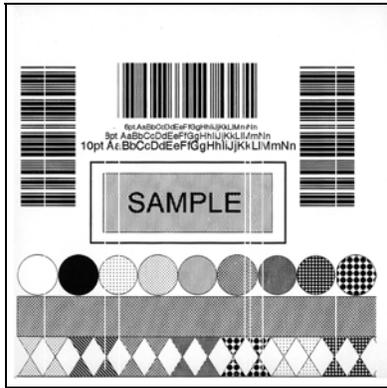
**Note:** Streaks can indicate a dirty or faulty printhead.
