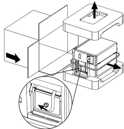
D. Place the printer in an upright position and remove the packing foam, bag, and tape.
