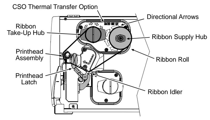
**Note:** Coating Side In and Coating Side Out ribbons are NOT interchangeable.
