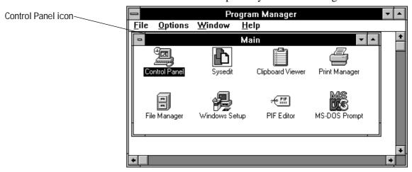
☐ In the "Control Panel" window, open the "Printers" option by double-clicking the icon.
