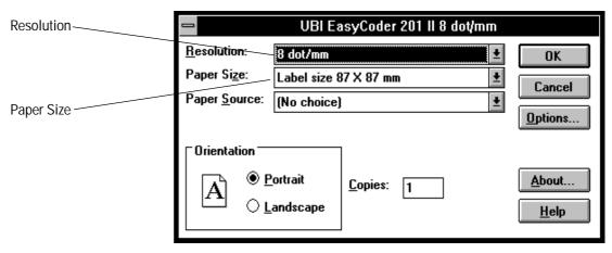
• **Resolution** is information only and shows the printhead density for the selected printer:
