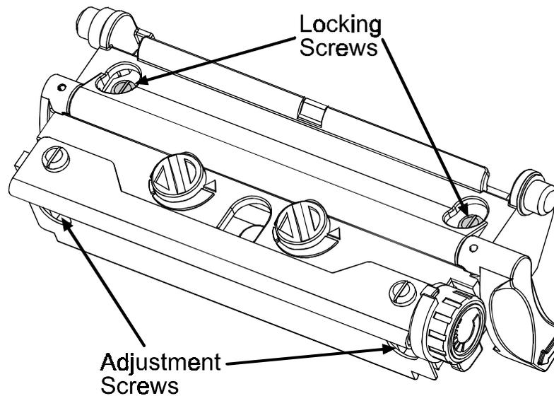
**Note:** When the Locking Screws are 'snug', turning the Adjustment Screws counter-clockwise will not move the printhead outward. If you have adjusted the printhead too far inward, restart the entire procedure.
