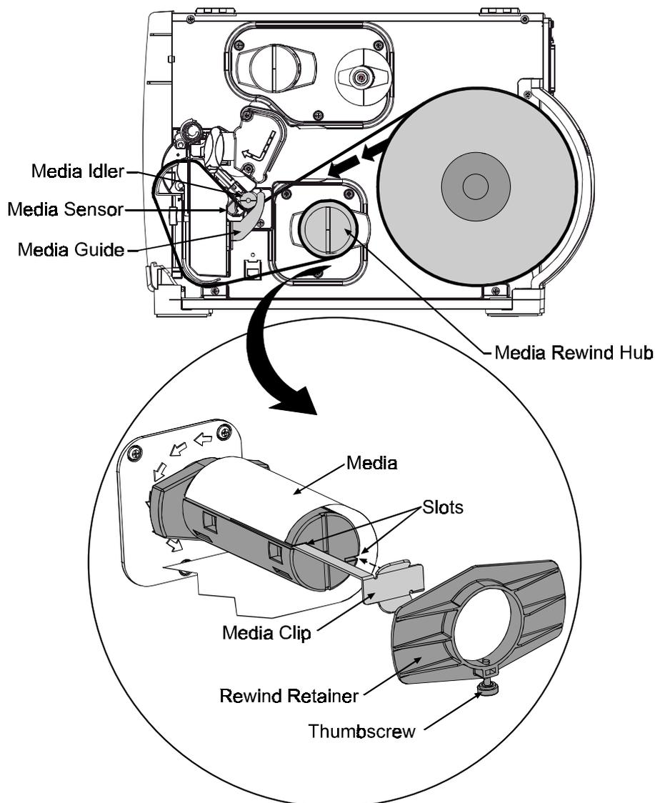
➡ After finishing, close the Access Cover, then push and hold the FEED key for 4 seconds to secure the backing material and calibrate the TOF.
