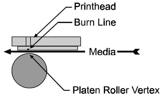
When media with a different thickness or rigidity is used (e.g., heavy tag stock), an adjustment may be needed *if* the print quality has been adversely affected. Generally, thicker media requires a slight forward adjustment of the printhead while thinner media requires a backward adjustment to compensate for the change in the burn line to vertex relationship.
