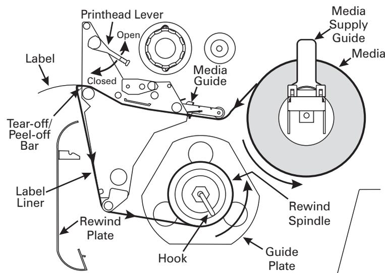
**Figure 2-6. Peel-Off Mode Loading**
