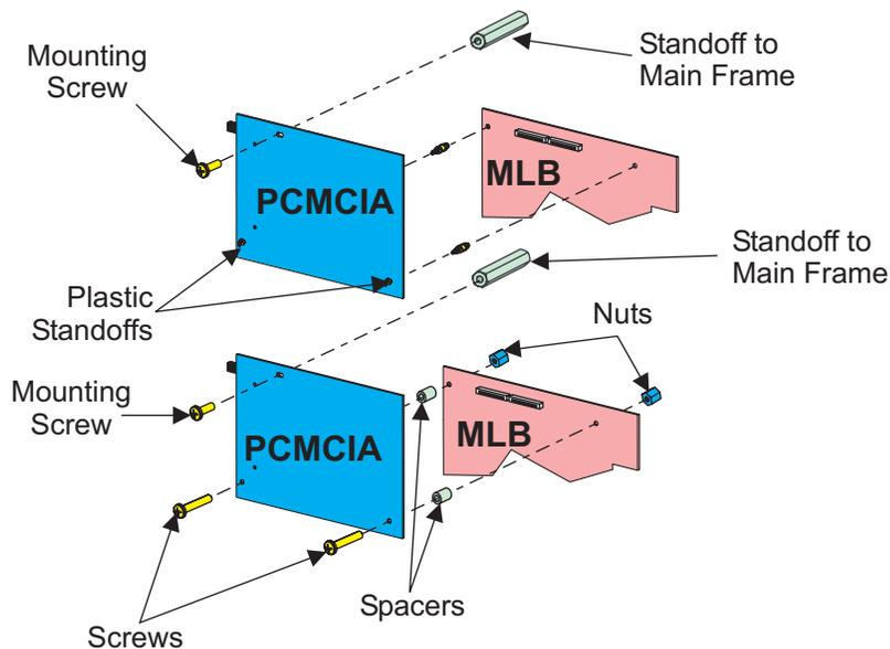
**Figure 4-89. Standoffs****Install the Wireless PCMCIA or PCMCIA Option Board Assemblies**
