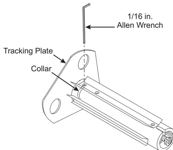
**Figure 4-63. Adjust the Rewind Spindle Assembly Position**
