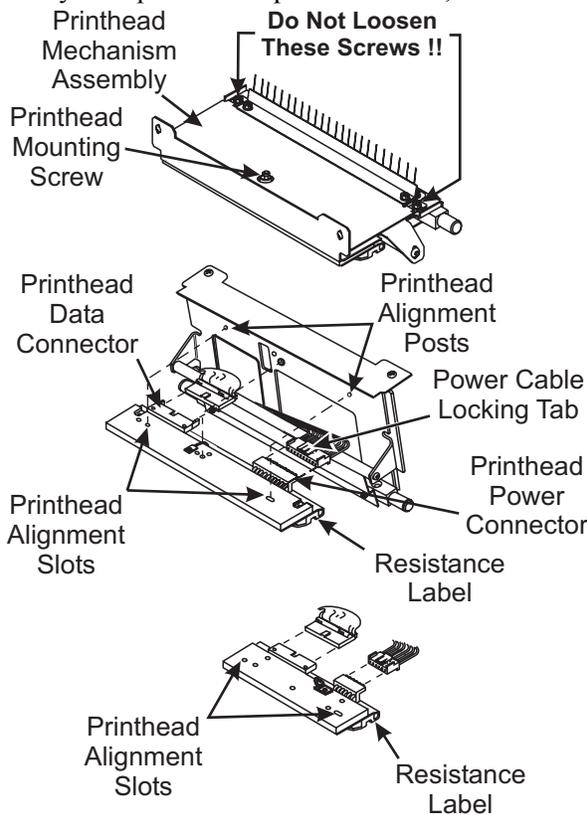
Figure 4-18. Printhead Replacement
