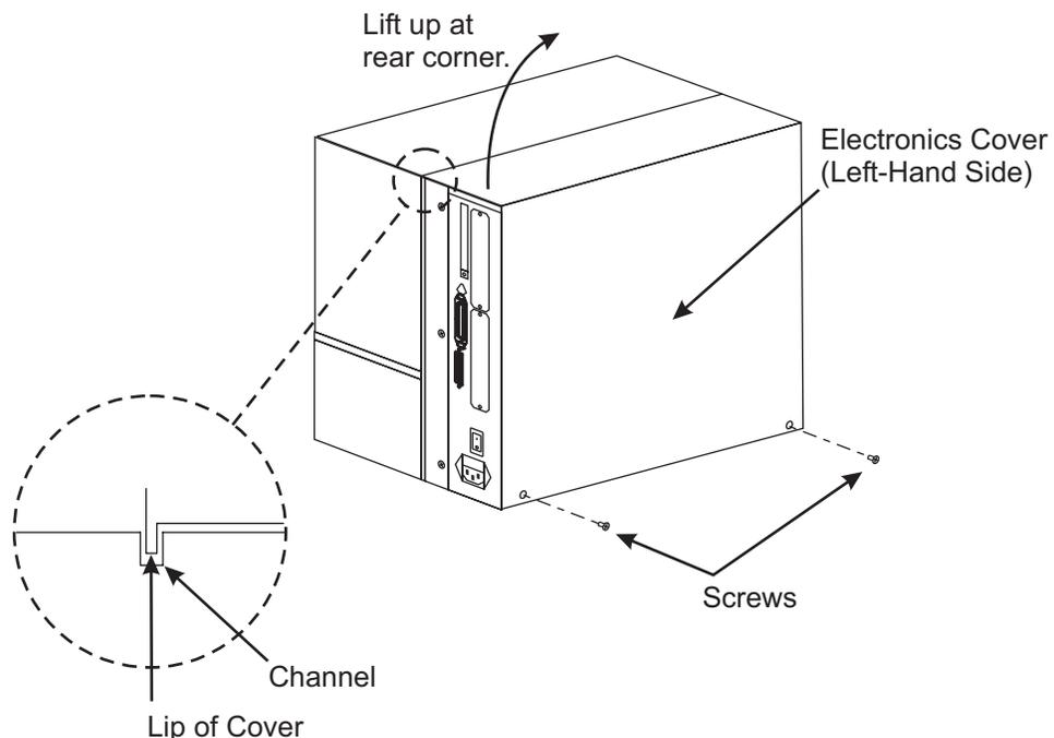
**Figure 4-7. Remove and Install the Electronics Cover**
