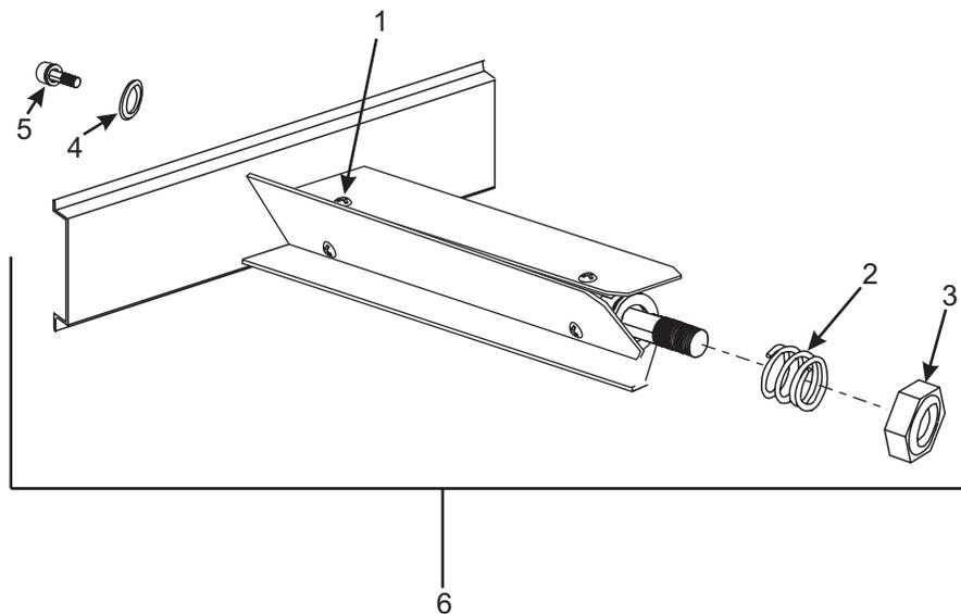
**Figure 5-8. Optional Media Supply Spindle**
