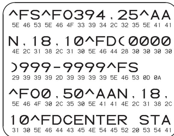
Figure 3-5. Communications Diagnostics Self Test
