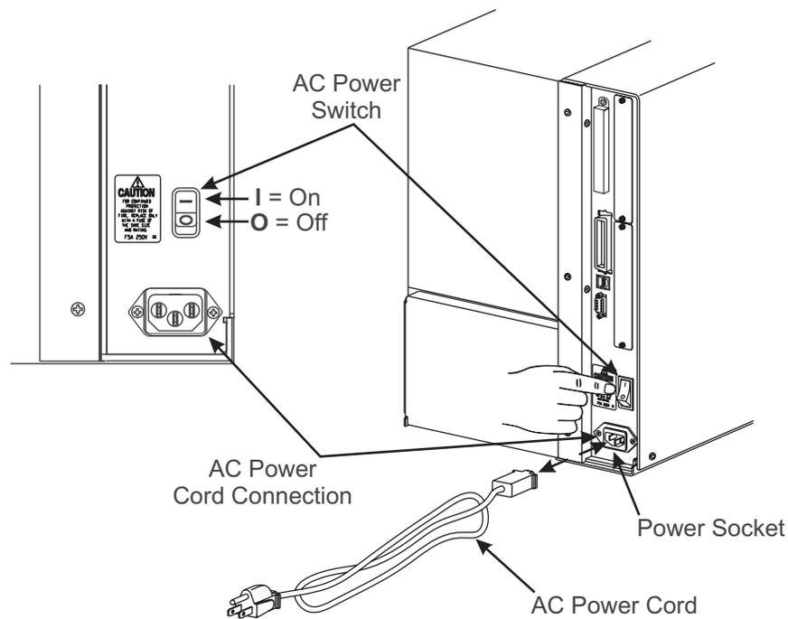
**Figure 4-5. Power Cord Removal and Installation**
