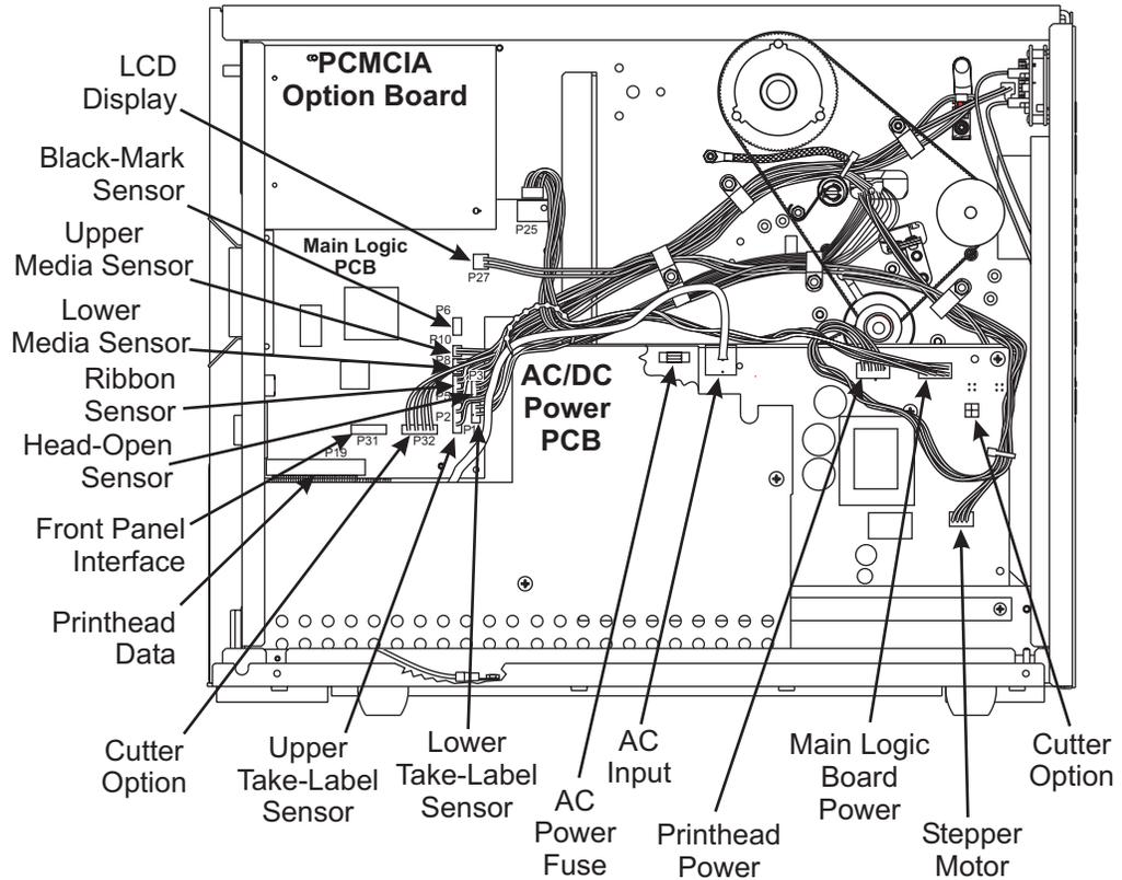
Figure 4-75. PCB Location and Interconnections
