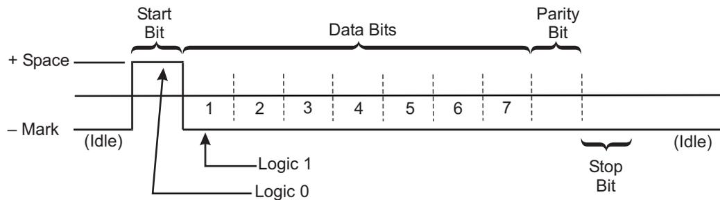
**Figure 1-10. RS-422 and RS-485 Signaling**
