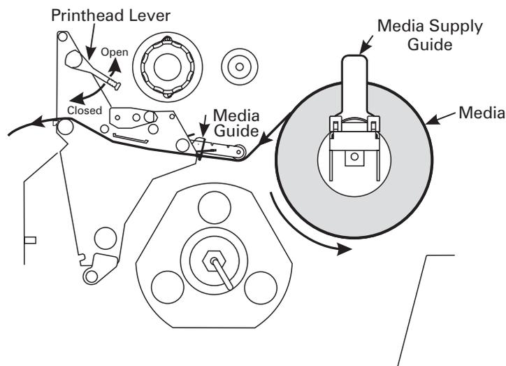
**Figure 2-5. Roll Media Loading Tear-Off Mode**
