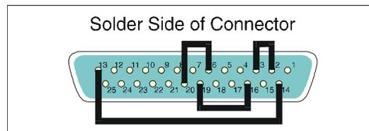
Figure 3-6. Parallel Loopback Connector
