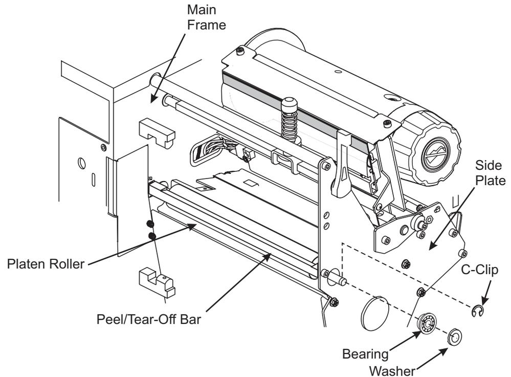
**Figure 4-51. Remove the Side Plate**
