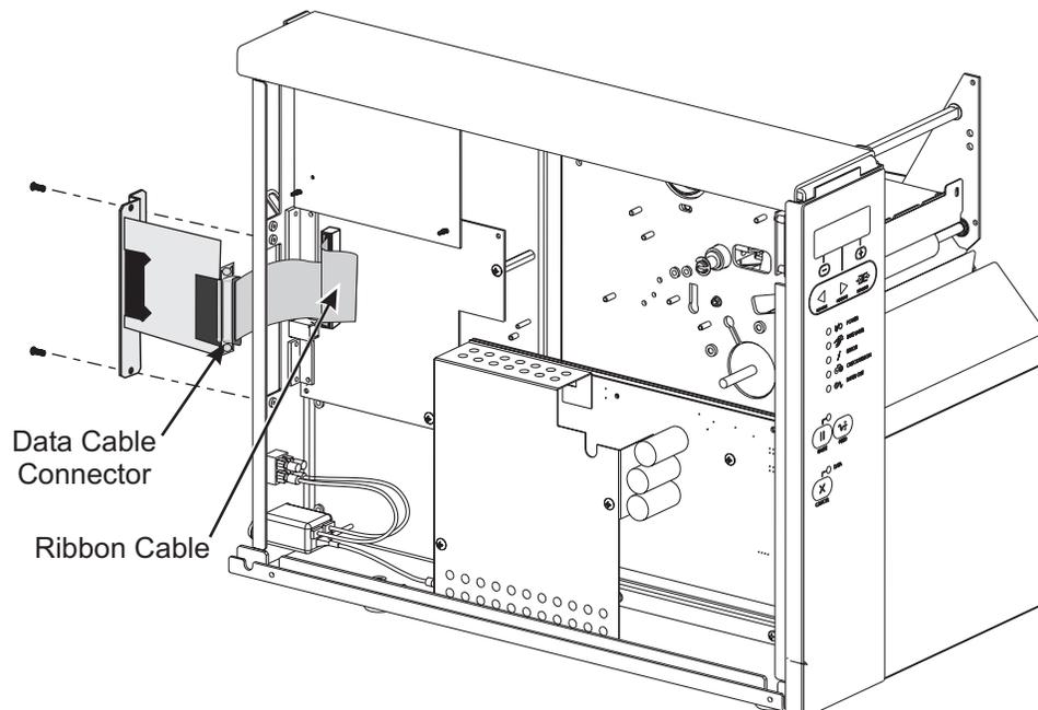
**Figure 4-72. Coax Communications Interface Board Installation**
