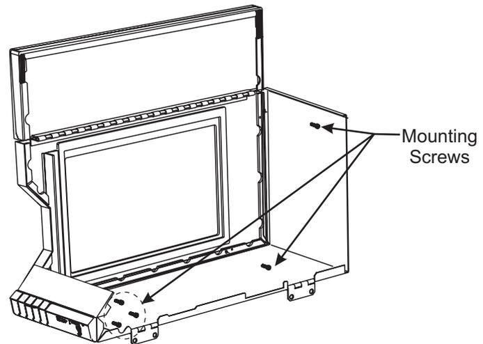
**Figure 4-59. Install Bifold Door**
