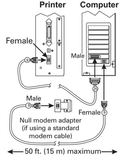
Figure 1-6. Serial Data Port
