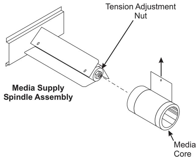
**Figure 4-58. Adjust Spindle Tension**
