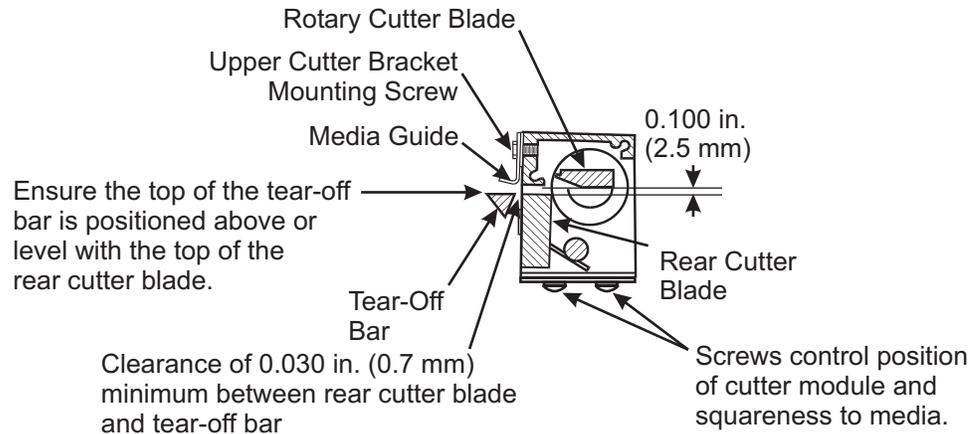
Relative position of the rotary cutter blade when the drive link assembly is stopped by the optical sensor, when the power is On (I) in Cutter Mode.
