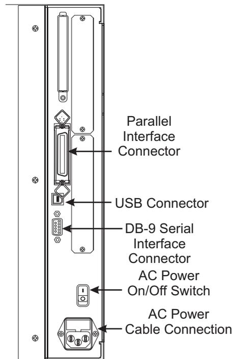
**Figure 1-4. Interface Connections**
