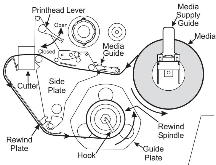
**Figure 2-9. Rewind Mode w/Cutter Loading**
