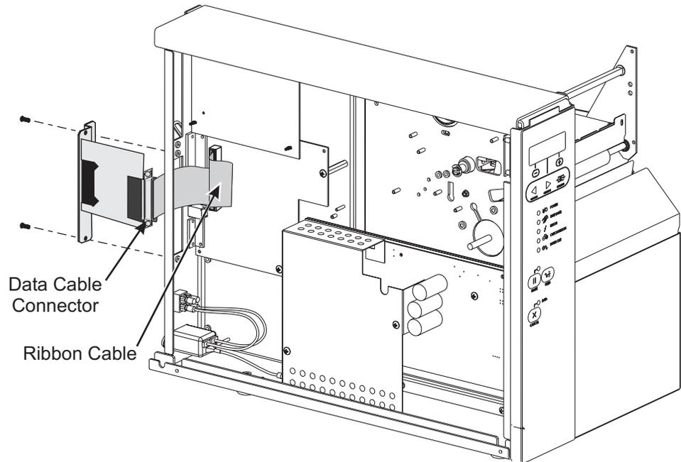
**Figure 4-71. Twinax Interface Board Installation**
