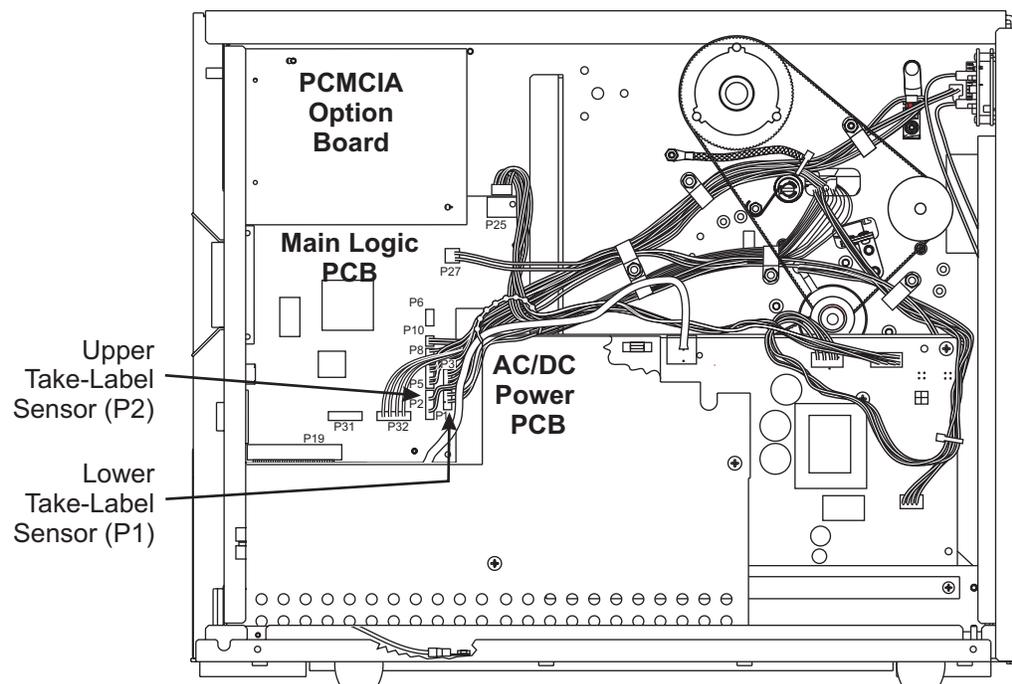
**Figure 4-62. Take-Label Sensor Connections**
