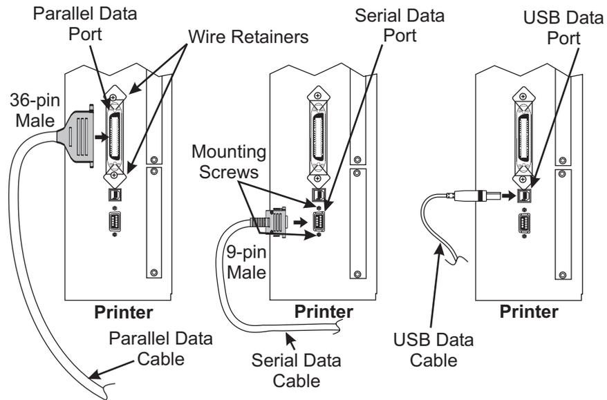
**Figure 4-6. Remove and Install the Data Cables**
