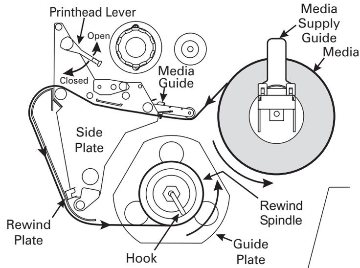
**Figure 2-7. Rewind Mode without Cutter Option**
