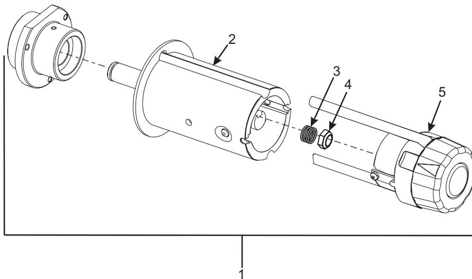
Figure 5-9. Ribbon Take-Up Spindle Assembly
