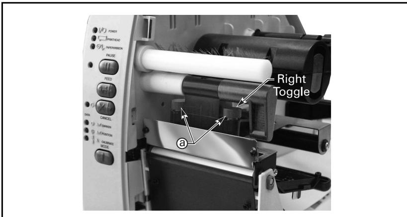
**Figure 23. Toggle Pressure Adjustment**
