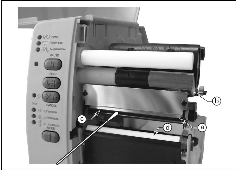
**Figure 16. Printhead and Platen Roller Cleaning**
