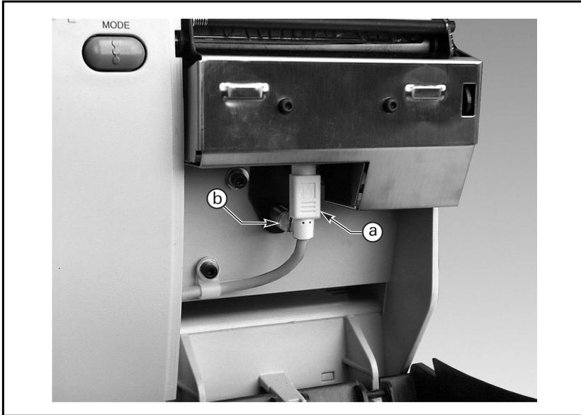
**Figure 18. Cutter Cable Connector Removal**
