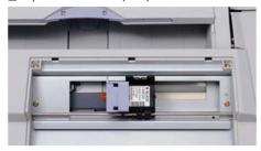
Note: Imprinter is the device for recognizing scanned documents by imprinting numbers on each document. fi-486PRFR enables users to store image data with imprint numbers on.
