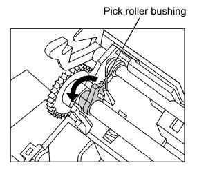
3) Remove the Pick roller while lifting it up in the direction of the arrow.
