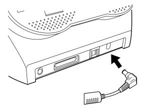
3. Insert the AC cable into the outlet.
