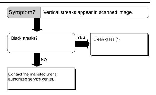
\*) For details on how to clean Sheet guide(A white portion) and glass, see "5.2 Cleaning the ADF."
