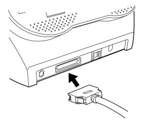
2. Connect the connector on the other end of the cable to the personal computer.
