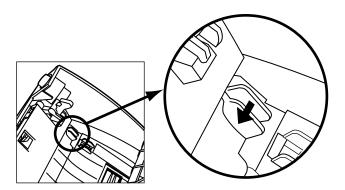
**2)** Rotate the Pick roller bushing in the direction of the arrow.
