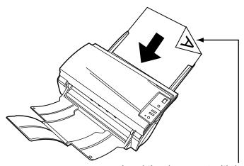
Load the document with its front side facing the ADF paper chute.(face down)
