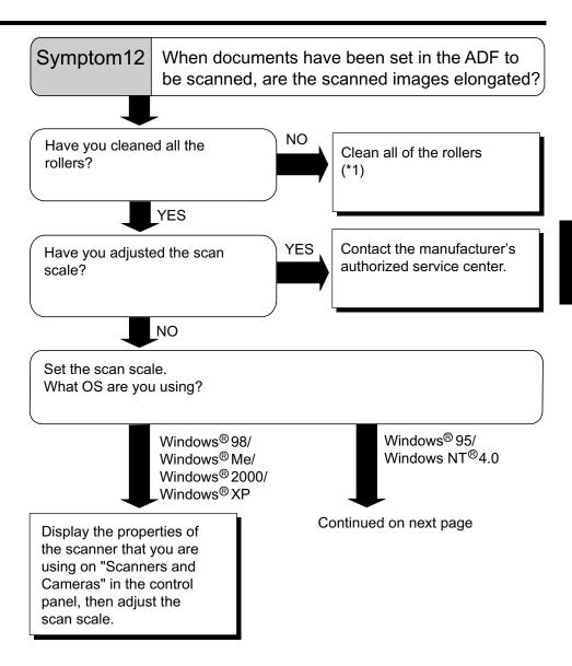
\*) For details on how to clean the rollers, see "5.2 Cleaning the ADF."
