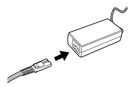
2. Connect the connector of AC adapter to the DC inlet of the scanner.
