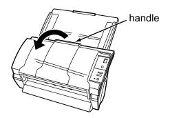
2. Lift the paper stop and swing forward by inserting your fingertips into the indentations on the scanner as shown in below figure.
