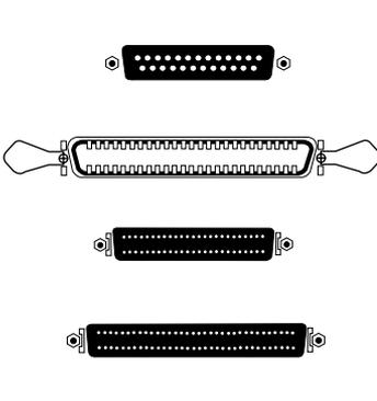
Possible shapes of the SCSI connector on the computer
