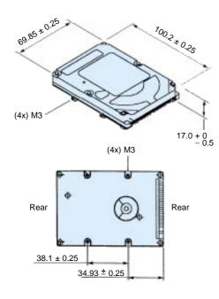
The recommended mounting screw torque is  $3 \pm 0.5$  kgf.cm.
