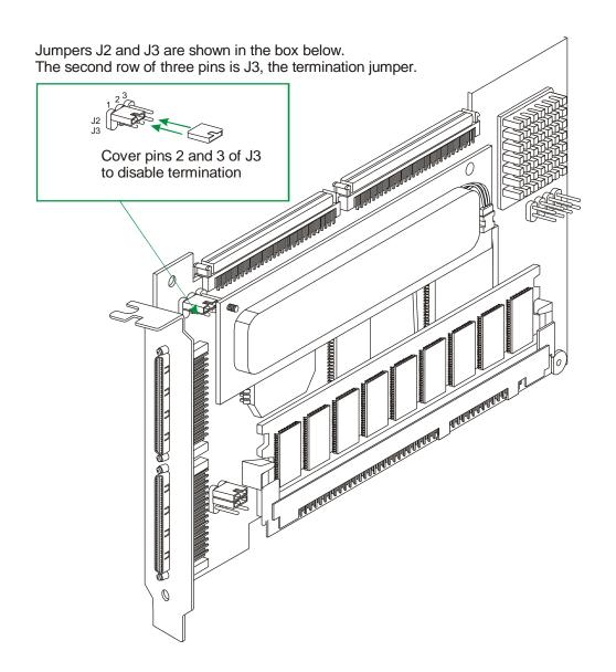
Setting Jumper J3 on the NetRAID-2M Controller to Disable Termination
