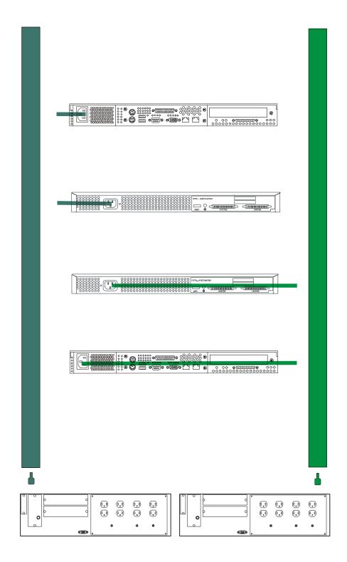
**Power Cabling to Separate Power Circuits**
