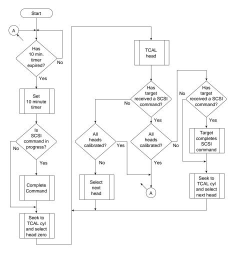
Figure 3. OEM interruptible thermal calibration implementation
