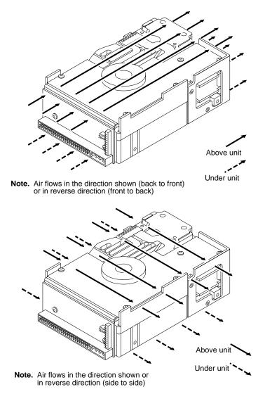
Figure 6. Air flow (ST15150N shown)
