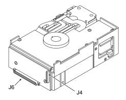
Figure 23. ST15150WC/DC drives option header locations
