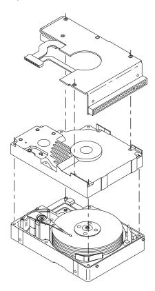
Figure 2. Barracuda 4 disc drive (exploded view)
