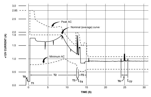
Figure 14. Typical Barracuda 4 drive +12V current profile
