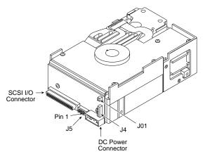
Figure 29. ST15150W/WD drives physical interface
