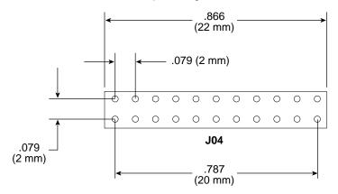
Figure 26. ST15150N/ND drives configuration select header specification
