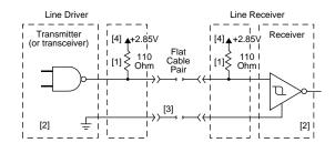
Figure 31. Single-ended transmitters and receivers
