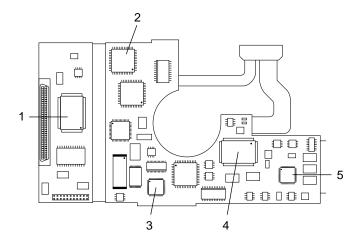
Figure 11. JYHX temperature measurement locations
