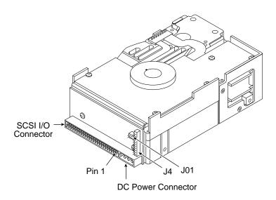
Figure 19. ST15150N/ND drives option header locations
