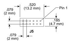
Figure 27. ST15150W/WD drives configuration select header specification
