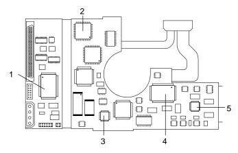
Figure 9. MYHX temperature measurement locations
