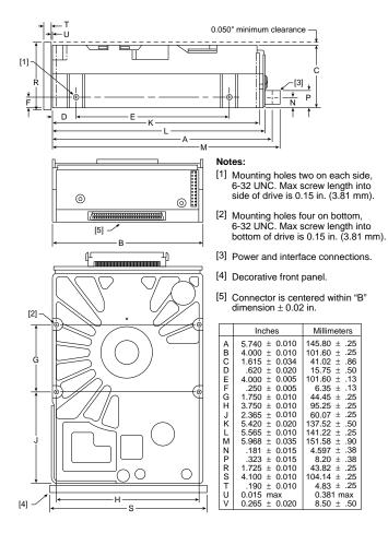
Figure 17. Mounting configuration dimensions for WC/DC drives
