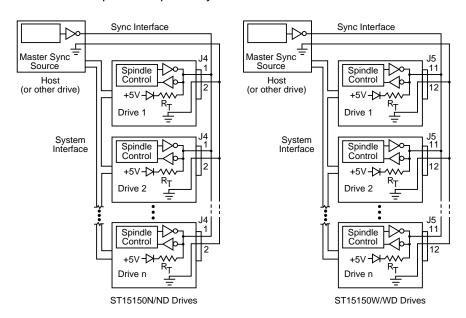
Figure 4. Synchronized drive interconnect diagram
