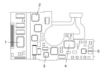
Figure 12. KYHX temperature measurement locations
