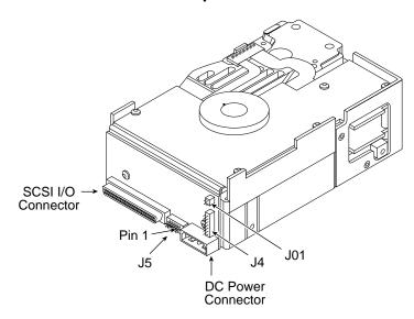
Figure 21. ST15150W/WD drives option header locations
