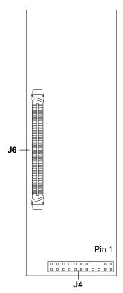
Figure 24. ST15150WC/DC drives option select connectors
