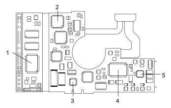
Figure 8. LYHX temperature measurement locations
