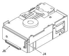
Figure 30. ST15150WC/DC drives physical interface
