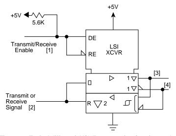
Figure 32. Typical differential I/O line transmitter/receiver and terminators
