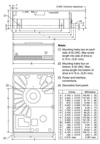
Figure 15. Mounting configuration dimensions for N/ND drives
