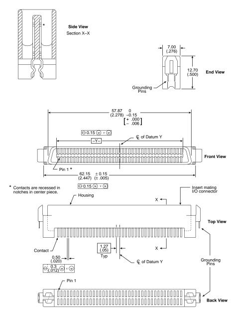
Figure 35. SCA SCSI device connector
