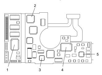
Figure 10. NYHX temperature measurement locations
