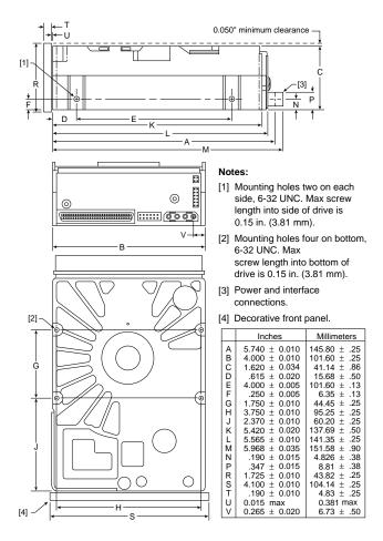
Figure 16. Mounting configuration dimensions for W/WD drives
