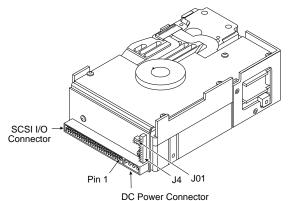
Figure 28. ST15150N/ND drives physical interface
