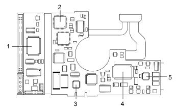
Figure 7. AYHX temperature measurement locations
