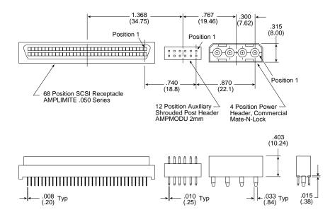
Figure 34. Wide SCSI device connector
