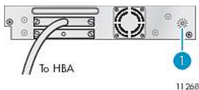
Figure 13 Tape drive LED
