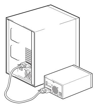
Figure 26 SCSI termination on a single Ultrium tape drive
