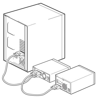
Figure 27 SCSI termination in daisy-chained external drives
