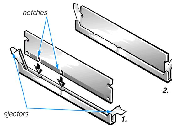
**Figure 8-5. Installing a DIMM**
