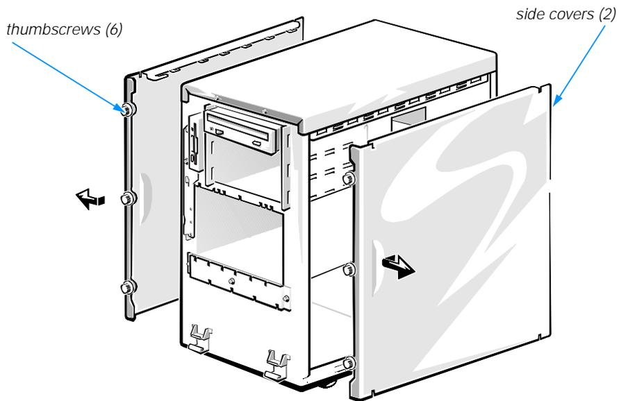
**Figure 7-3. Removing the Computer Covers**
