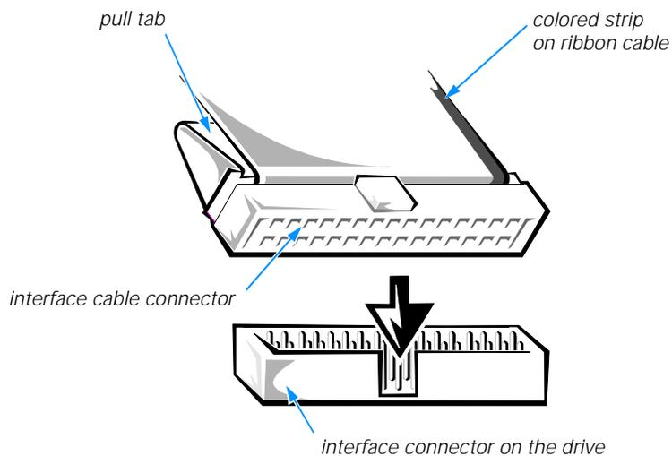
**Figure 9-3. Header Interface Connector**
