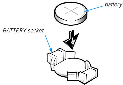
**Figure 8-11. Installing the Battery**
