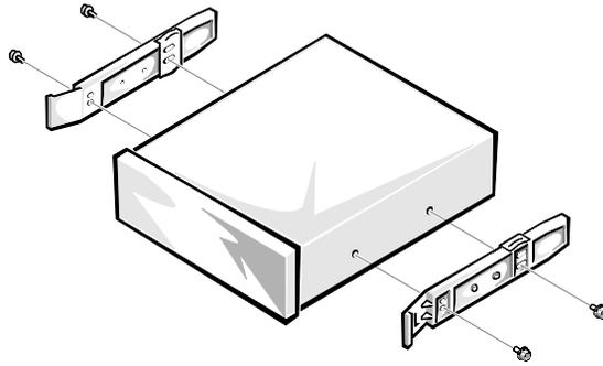
**Figure 9-6. Attaching Drive Rails**
