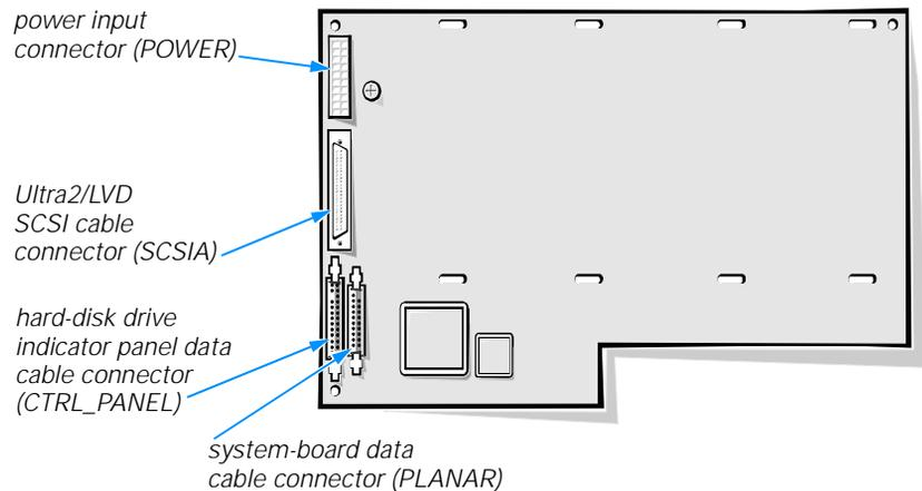
**Figure 10-7. Connectors on the 1 x 6 Hot-Pluggable SCSI Backplane Board**
