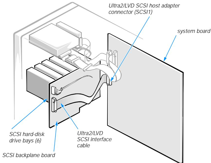
**Figure 10-1. Hard-Disk Drive Hardware (1 x 6 Hot-Pluggable SCSI Backplane Board Shown)**
