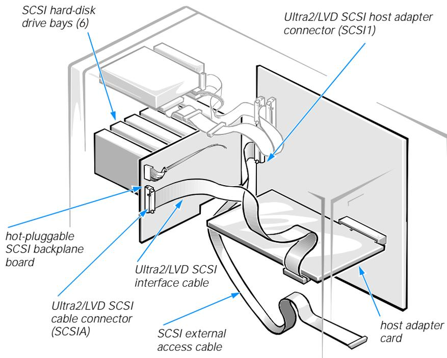
**Figure 10-5. Cable Configuration for a Dell PowerEdge Expandable RAID Controller Host Adapter Card**
