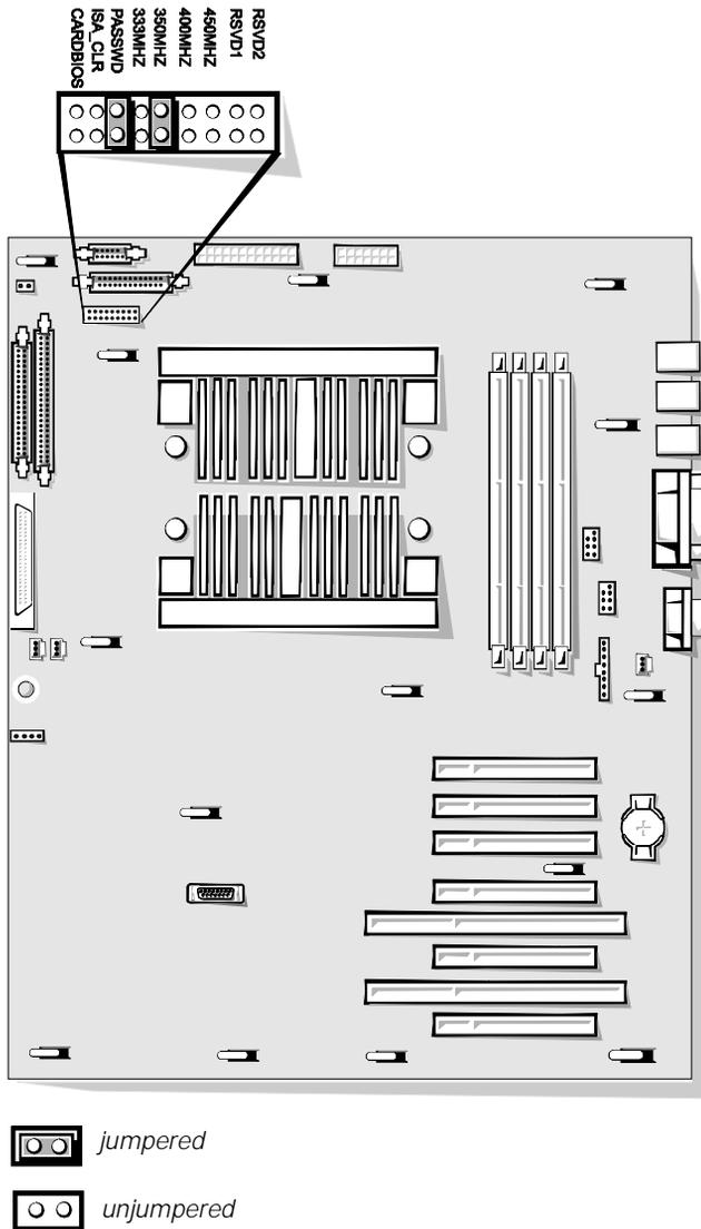
**Figure B-1. System Board Jumpers**
