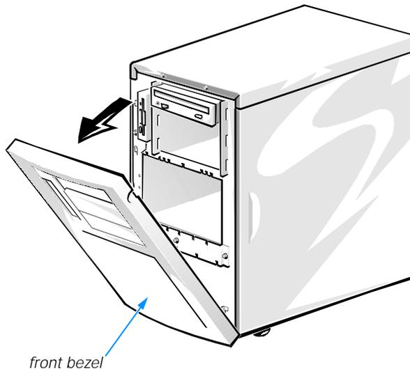
**Figure 7-2. Opening the Front Bezel**
