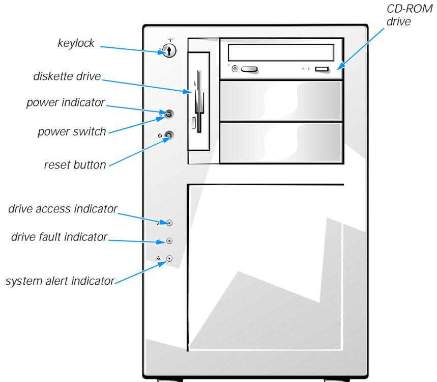
**Figure 2-2. Front Panel Features**
