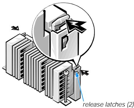
**Figure 8-8. SEC Cartridge Release Latches**
