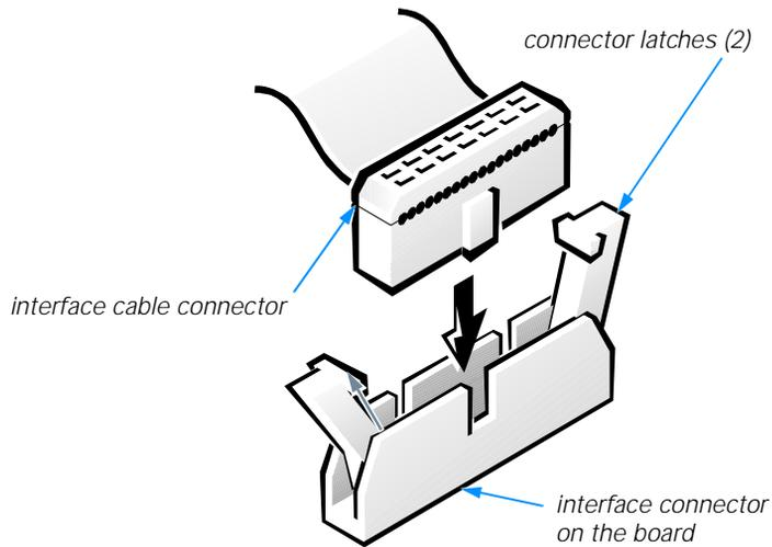
**Figure 9-4. Latching Interface Connector**
