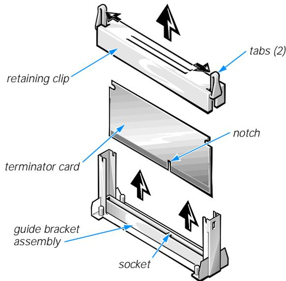
**Figure 8-7. Removing a Terminator Card**
