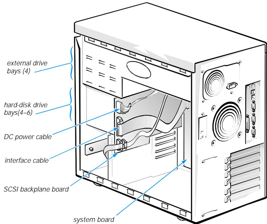
**Figure 7-4. Inside the System (Right-Side View)**
