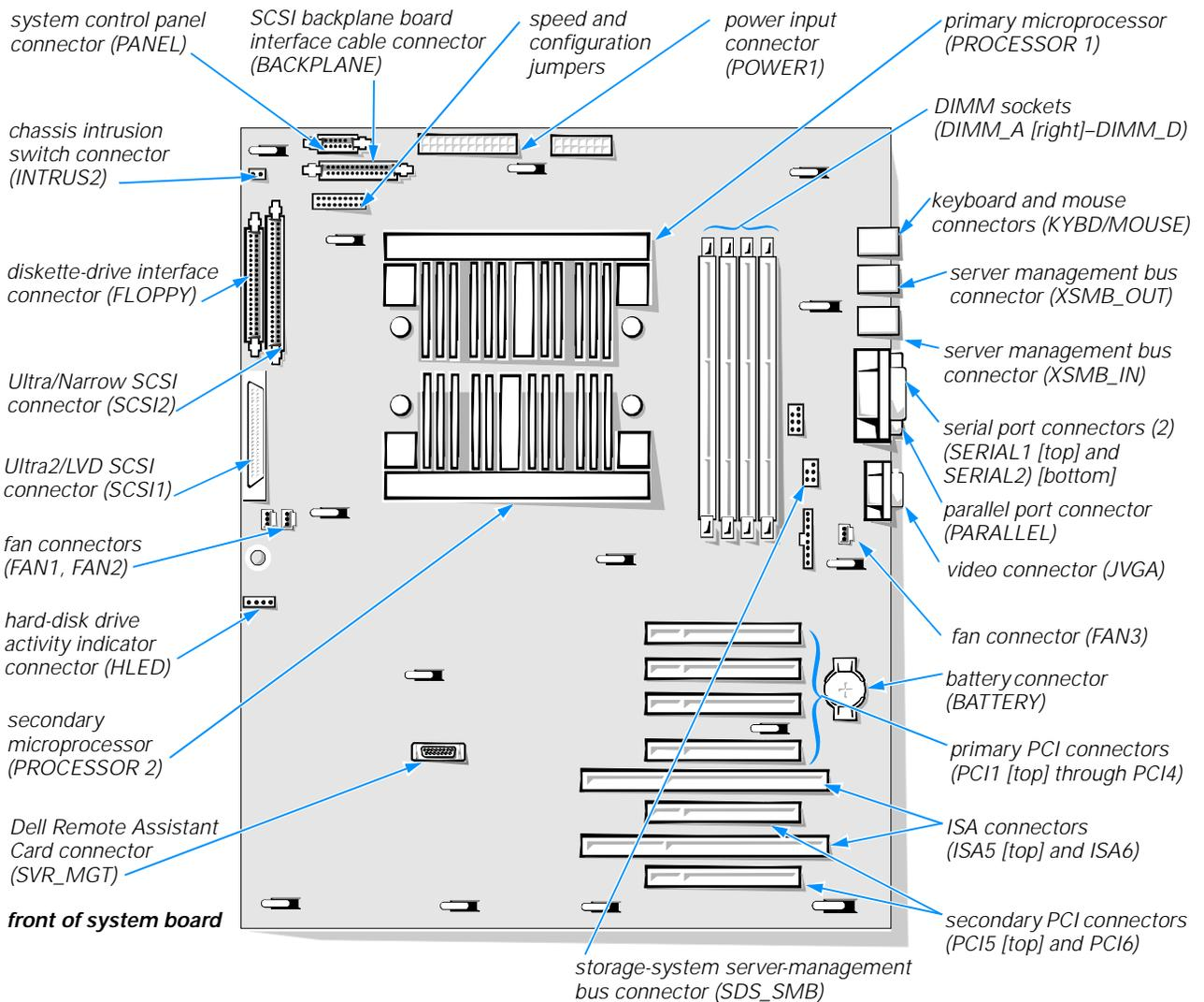
**Figure 8-1. System Board Features**
