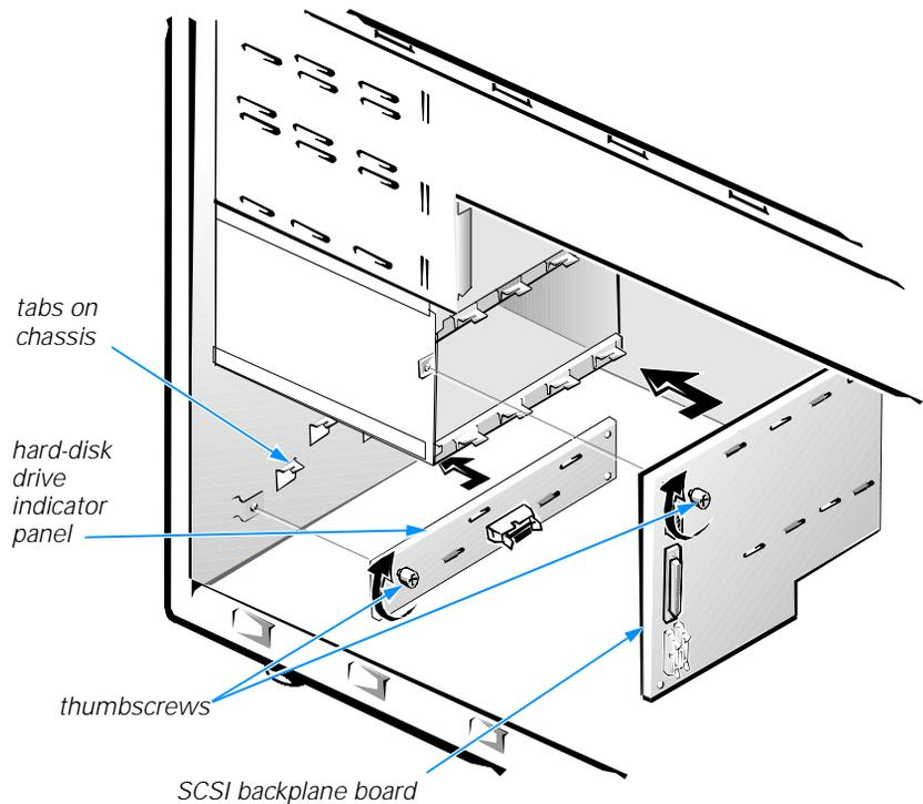
**Figure 10-6. Installing the 1 x 6 Hot-Pluggable SCSI Backplane Board and Hard-Disk Drive Indicator Panel**
