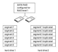
If a drive failure occurs, subsequent read and write operations are directed to the surviving drive. A replacement drive can then be rebuilt using the data from the surviving drive. Also, because data is duplicated on both drives, two 120-GB RAID level 1 drives collectively have a maximum of 120-GB on which to store data.
