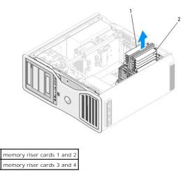
6. Disconnect the power cables from memory riser cards 3 and 4.
