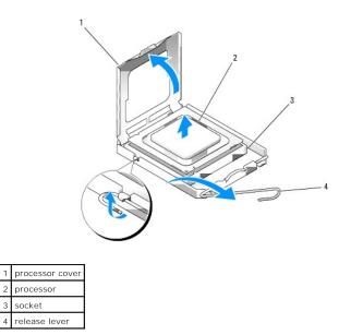
7. Orient the front and rear alignment notches on the processor with the front and rear alignment notches on the socket.
