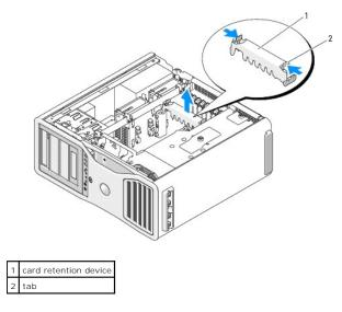
4. Press down the tab on the top of the card retainer at the appropriate card slot and pivot the card retainer back through the chassis wall.
