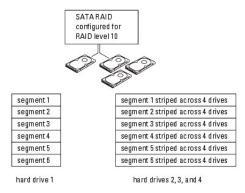
If a drive failure occurs, subsequent read and write operations are directed to the other surviving drives. A replacement drive can then be rebuilt using the data from the surviving drives. Also, because data is duplicated on the primary and additional drives, four 120-GB RAID level 1 drives collectively have a maximum of 240-GB on which to store data.
