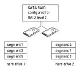
Another advantage of a RAID level 0 configuration is that it utilizes the full capacities of the drives. If you have two 120-GB drives installed, you have 240 GB on which to store data.
