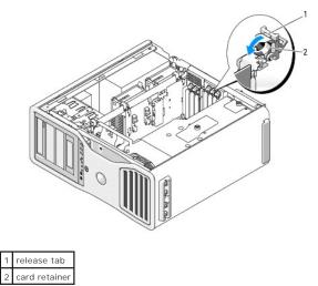
13. Press the card retention device back into its original position; push it down until it clicks into place.
