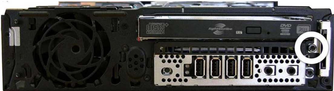
Figure 9-20 Removing the card reader screw
