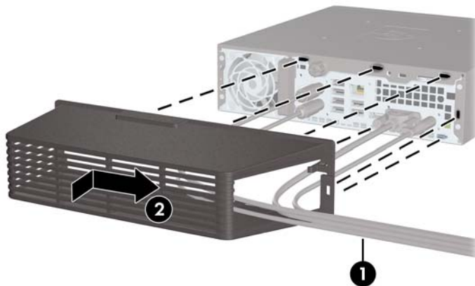
Figure 9-35 Installing a port cover
