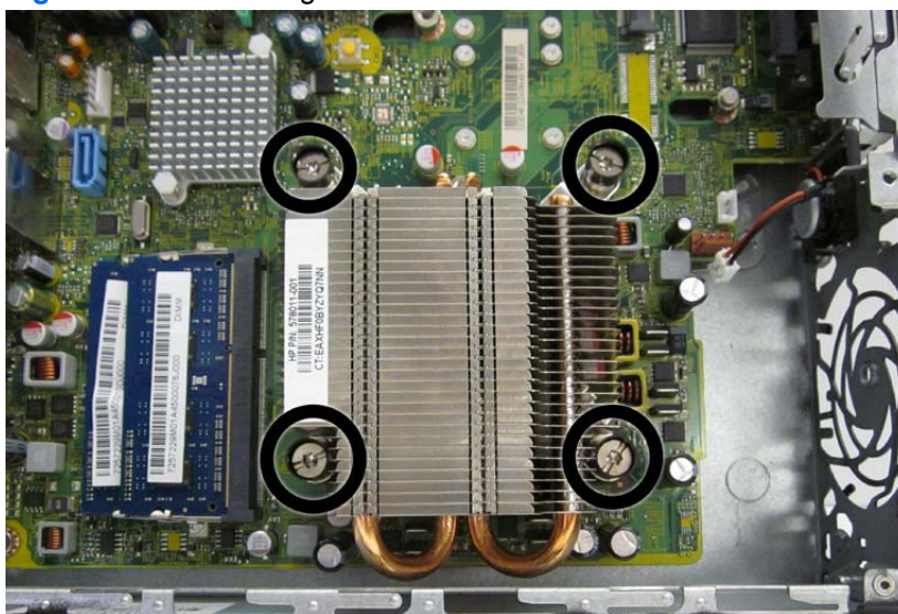
Figure 9-23 Loosening the heat sink screws
