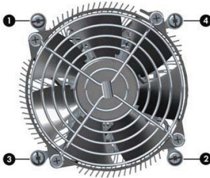
Figure 6-44 Loosening the fan sink screws
