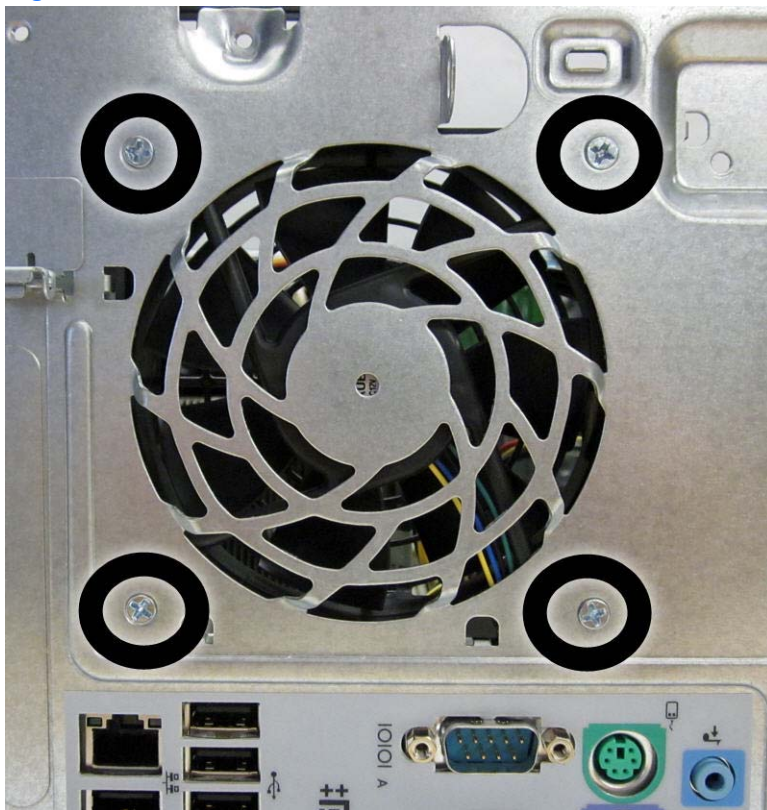
Figure 7-32 Rear fan screws
