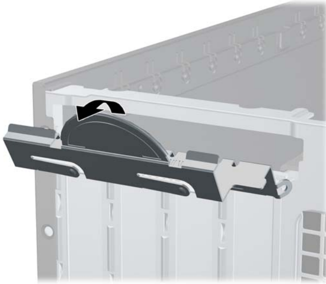
Figure 8-5 Opening the expansion slot retainer
