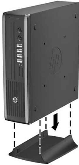
Figure 9-34 Placing the computer on the stand
