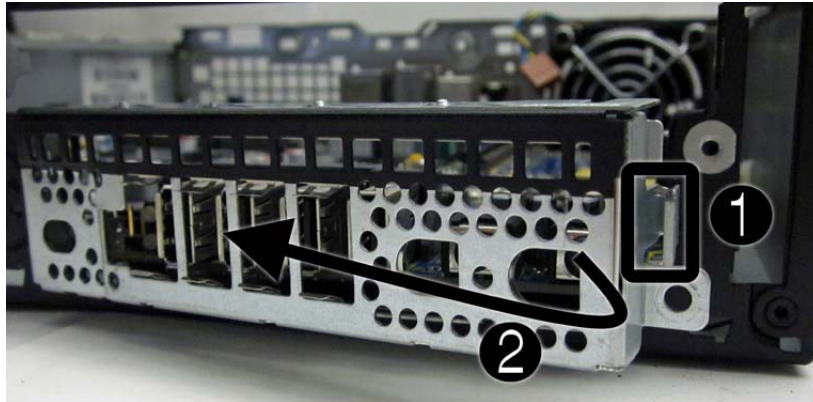
Figure 9-30 Removing the I/O panel
