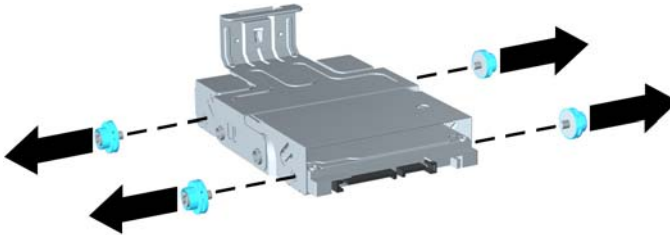
Figure 9-14 Removing the guide screws
