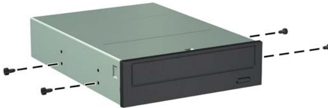
Figure 8-16 Installing Guide Screws in the Optical Drive
