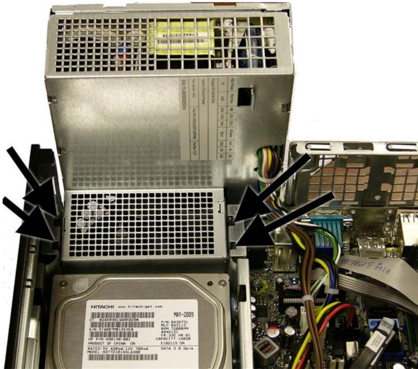
Figure 8-38 Removing the power supply
