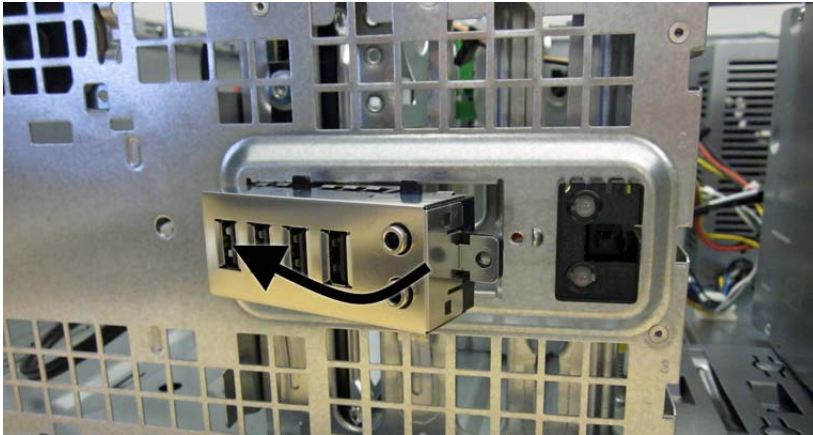
Figure 6-40 Removing the front I/O, USB, power switch assembly
