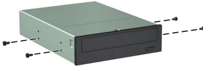
Figure 7-17 Installing Guide Screws (Optical Drive Shown)
