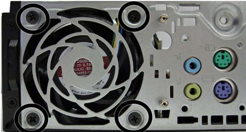
Figure 9-32 Removing the rear fan screws
