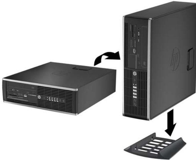
Figure 8-40 Changing from Desktop to Tower Orientation
