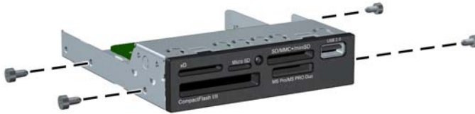
Figure 8-20 Installing Guide Screws (Media Card Reader Shown)
