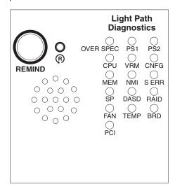
To acknowledge a system error but not take immediate action, press the remind button to place the server in Remind mode. When the server is in Remind mode, the system-error LED on the front of the server flashes. If a new failure occurs, the system-error LED is lit again.
