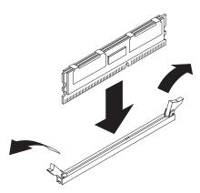
To install a DIMM, complete the following steps:
