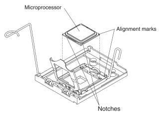
d. Align the microprocessor with the socket (note the alignment mark and the position of the notches); then, carefully place the microprocessor on the socket. Close the microprocessor bracket frame.
