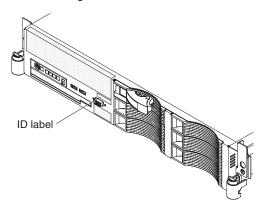
Note: This illustration shows a model with 3.5-inch serial-attached SCSI (SAS) hot-swap hard disk drives. Models with 2.5-inch SAS hot-swap hard disk drives are also available. The location of the ID label is the same on both model styles. This illustration might differ slightly from your hardware.
