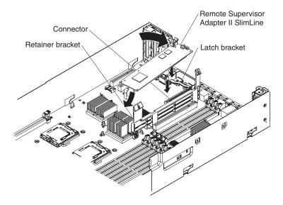
To install a Remote Supervisor Adapter II SlimLine, complete the following steps:
