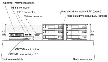
The following illustration shows the controls, light-emitting diodes (LEDs), and connectors on the front of the 2.5-inch model server.
