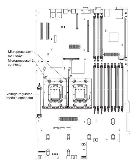
The following illustration shows how to install the second microprocessor on the system board.
