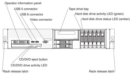
**Operator information panel:** This panel contains controls, LEDs, and connectors. The following illustration shows the controls, LEDs, and connectors on the operator information panel.
