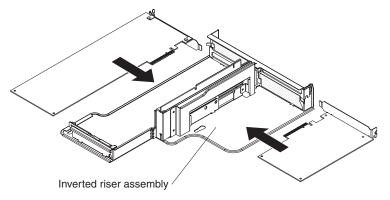
7. If you removed the PCI riser-card assembly to install the adapter, align the riser-card assembly with the release-tab posts, rear guides, and connector; then, press the PCI riser-card assembly *firmly* into the connector.
