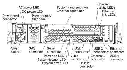
Power-cord connector (ac power supply only): Connect the power cord to this connector.
