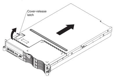
4. Lift the cover-release latch. Lift the cover off the server and set the cover aside.
