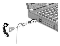
Wrap a computer security lock cable around an immovable object such as a table or locked drawer handle. Insert the lock into the notch and turn the key to secure the lock.
