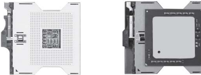
Figure 5-3. 604-pin Socket: Empty and with Processor Installed
