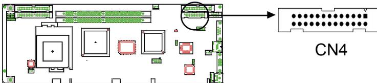
The parallel port is normally used to connect the CPU card to a printer. The onboard parallel port can be accessed through a 26-pin flat-cable connector, CN4. The card comes with an adapter cable which lets you use a traditional DB-25 connector. The cable has a 26-pin connector on one end and a DB-25 connector on the other, mounted on a retaining bracket. The bracket installs at the end of an empty slot in your chassis, giving you access to the connector.
