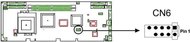
The PCA-6003 provides two USB (Universal Serial Bus) interfaces, which give complete Plug & Play and hot attach/detach for up to 127 external devices. The USB interface complies with USB Specification Rev. 1.0 and is fuse-protected.
