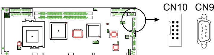
The PCA-6003 offers two serial ports, CN9 as COM1 and CN10 as COM2. These ports can connect to serial devices, such as a mouse or printers, or to a communication network.
