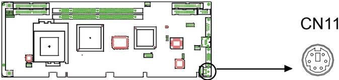
The PCA-6003 board provides a keyboard connector. A 6-pin mini-DIN connector (CN11) on the card mounting bracket supports single-board computer applications. The card comes with an adapter to convert from the 6-pin mini-DIN connector to a standard DIN connector and to a PS/2 mouse connector.
