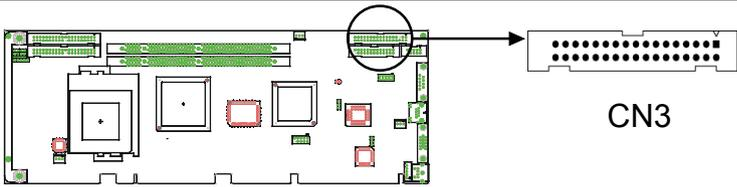
You can attach up to two floppy disk drives to the PCA-6003's onboard controller. You can use any combination of 5.25" (360 KB / 1.2 MB) and/or 3.5" (720 KB / 1.44/2.88 MB) drives.
