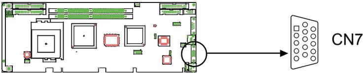
The PCA-6003 includes a AGP SVGA interface that can drive conventional CRT displays. CN7 is a standard 15-pin D-SUB connector commonly used for VGA. Pin assignments for CRT connector CN7 are detailed in Appendix B.
