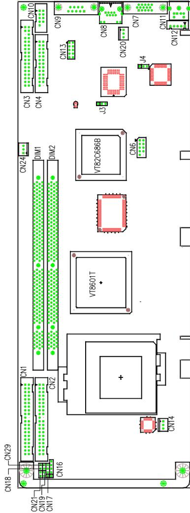
Figure 1-2: Board layout: jumper and connector locations
