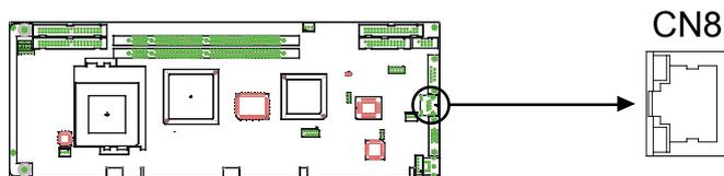
The PCA-6003 is equipped with a high-performance 32-bit PCI-bus Ethernet interface, which is fully compliant with IEEE 802.3/u 10/100 Mbps CSMA/CD standards. It is supported by all major network operating systems and is 100% Novell NE-2000 compatible. An onboard RJ-45 jack provides convenient 10/100Base-T RJ-45 operation.
