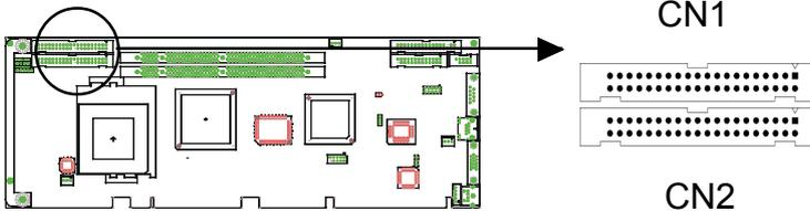
You can attach up to four IDE (Integrated Device Electronics) drives to the IDE connectors. The primary (CN1) and secondary (CN2) connectors can each accommodate two drives.
