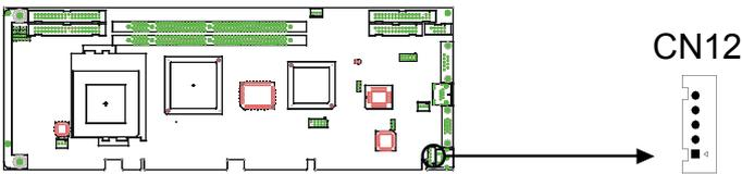
In addition to the PS/2 mouse/keyboard connector on the PCA-6003's rear plate, there is also an extra onboard external keyboard connector. This gives system integrators greater flexibility in designing their systems.
