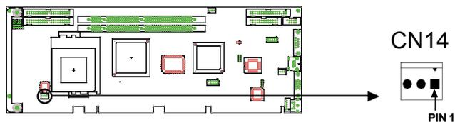
This connector supports a cooling fan with tachometer output.
