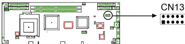
This connector supports the optional wireless infrared transmitting and receiving module. This module mounts on the system case. You must configure the setting through the BIOS setup (see Chapter 3).
