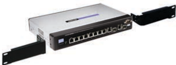
Attaching the Brackets
