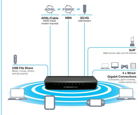
The NetComm Wireless NF5 is a future ready WiFi router that connects the home or office to super-fast broadband. Simply connect your fixed line modem to the Gigabit WAN port for instant Internet access - perfect for NBN/Fibre connections
