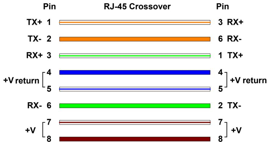
Pins 7 and 8 are used to carry power to the Canopy modules.
