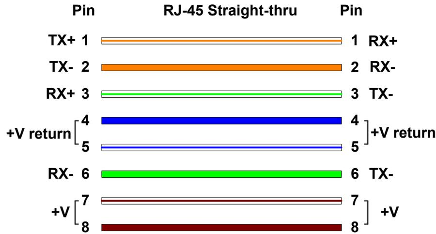
Pins 7 and 8 are used to carry power to the Canopy modules.
