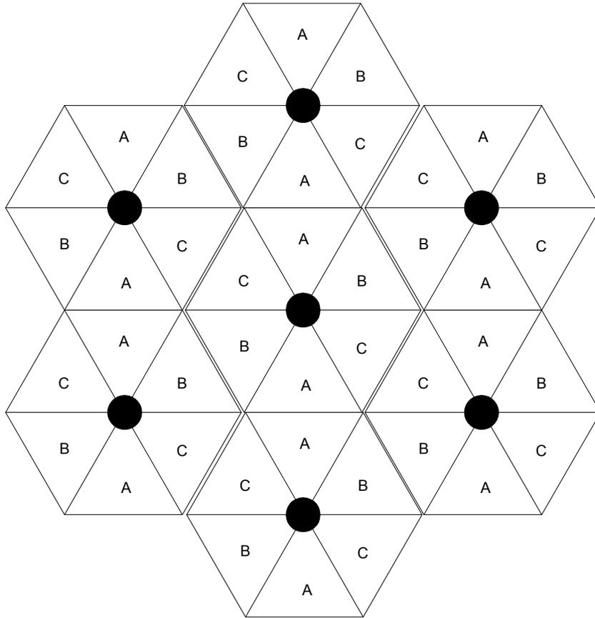
**Figure 27: Example layout of 7 Access Point clusters**
