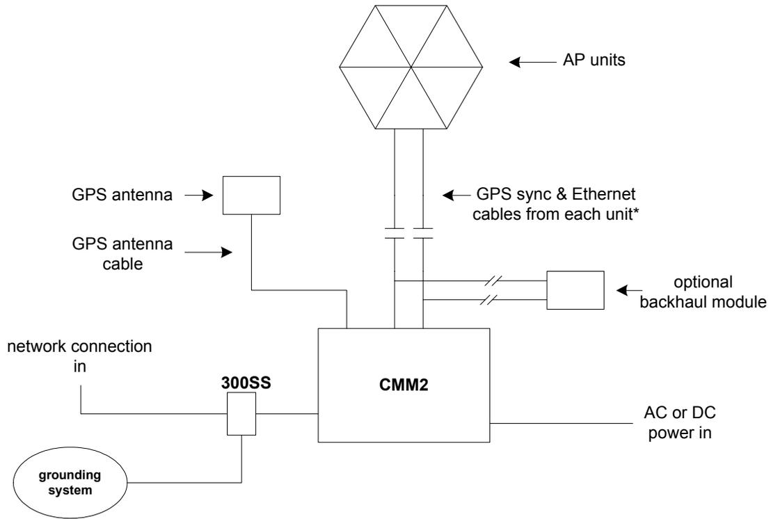
**Figure 4: Canopy system wiring**
