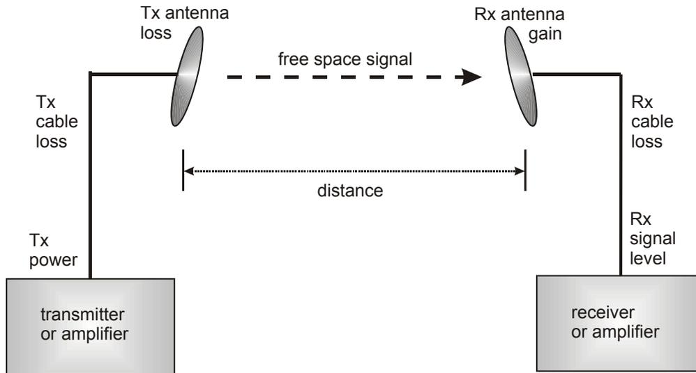
**Figure 22: Determinants in Rx signal level**
