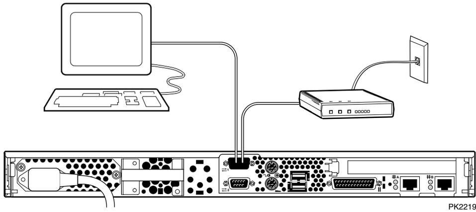
You can connect a terminal or a modem to the COM1 port, but not both at the same time. You use the terminal to set RMC parameters for the connection, then connect the modem. See Section 3.9.
