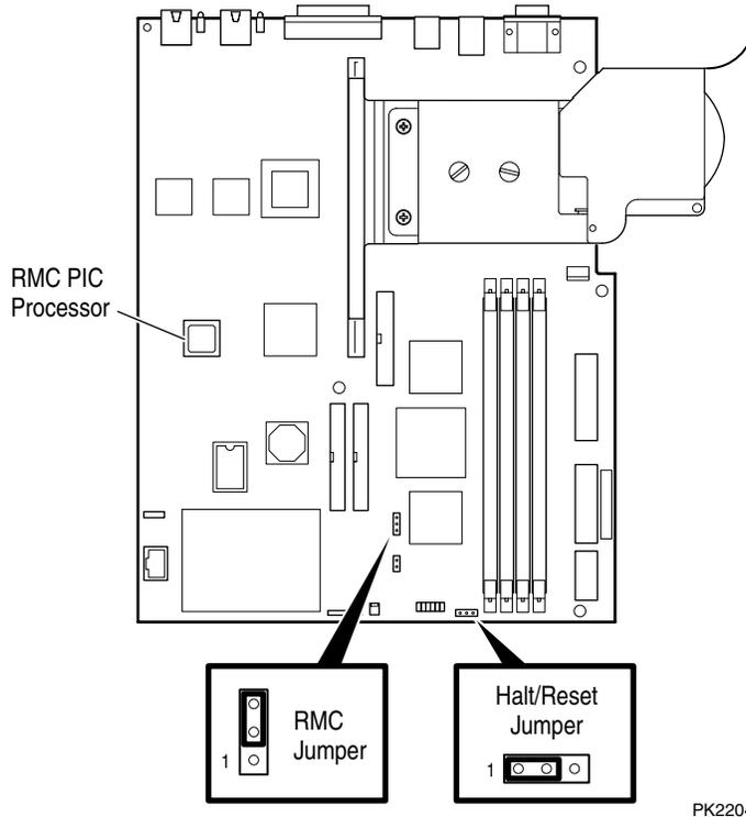
The RMC logic is implemented using an 8-bit microprocessor, PIC17C44, as the primary control device. The RMC PIC is programmed with code to control access to various environmental status bits.
