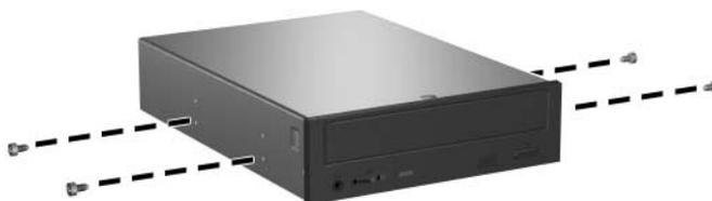
*Installing Guide Screws in the Optical Drive*
