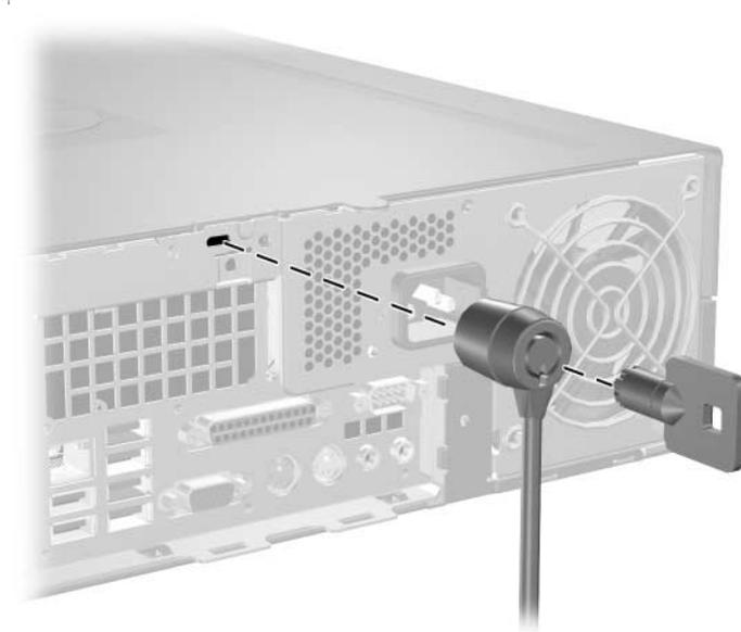
*Installing a Cable Lock*
