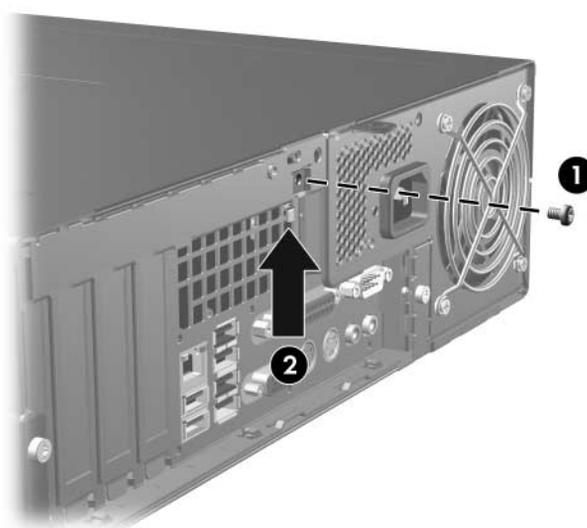
*Removing the Smart Cover Lock Screw*
