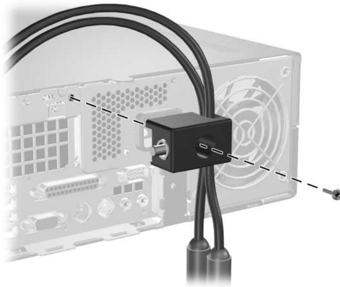
3. Insert the plug into the lock ❶ and push the button in ❷ to engage the lock. Use the key provided to disengage the lock.
