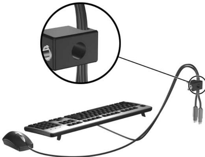
2. Screw the lock to the chassis using the screw provided.
