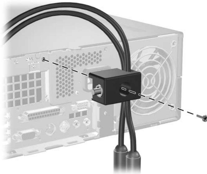
4. Insert the plug end of the security cable into the lock ❶ and push the button in ❷ to engage the lock. Use the key provided to disengage the lock.
