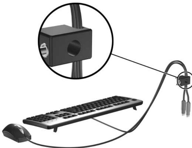
3. Screw the lock to the chassis using the screw provided.
