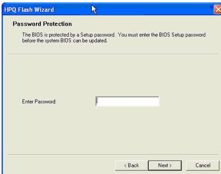
If you click the **Next** button, type the correct password (if needed), and have the appropriate rights, the application interrogates the current PC BIOS image and compares it to the BIOS image file (ROM.CAB) in the same directory as the Flashbin.exe. If the BIOS image file is not applicable to the PC, a warning message displays. If the image is applicable, HPQFlash displays the current BIOS and the BIOS version contained in the ROM.CAB file.
