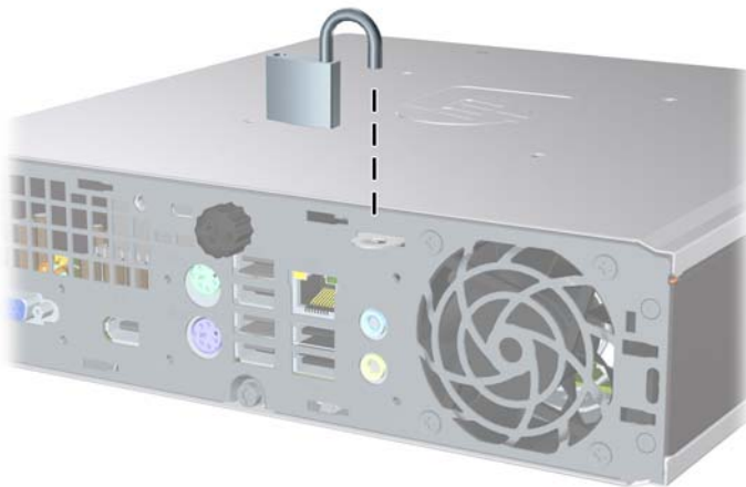
Figure C-3 Installing a Padlock
