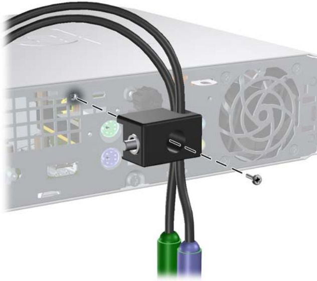
Figure C-6 Attaching the Lock to the Chassis
