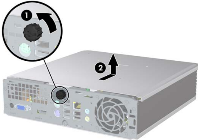
Figure 2-2 Removing the Computer Access Panel
