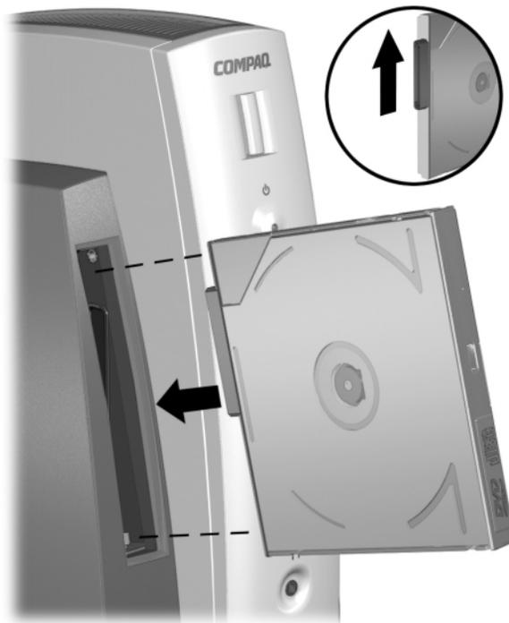
*Inserting a Drive into the MultiBay*
