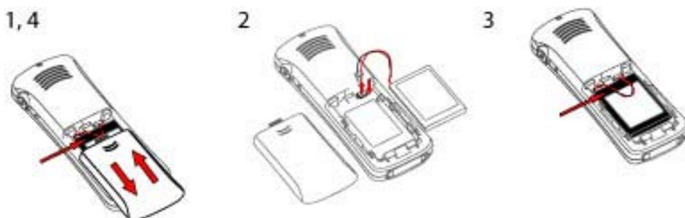
Figure 10: Battery replacement
