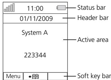
Figure 2: Example of a display in idle mode
