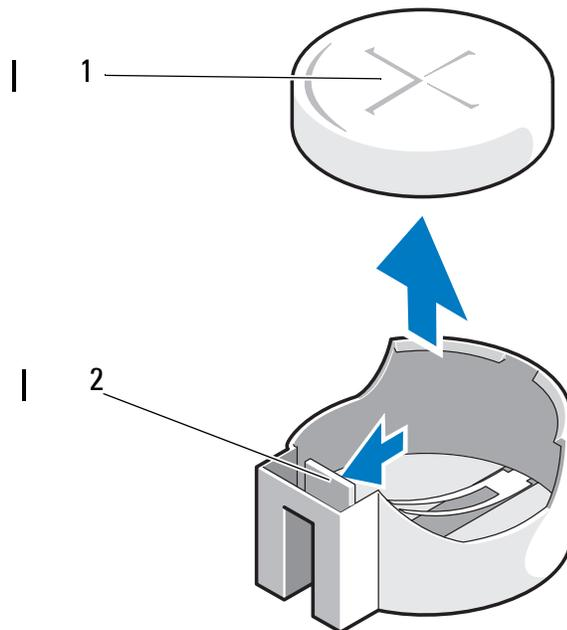
1 battery (positive side) 2 battery retention tab
