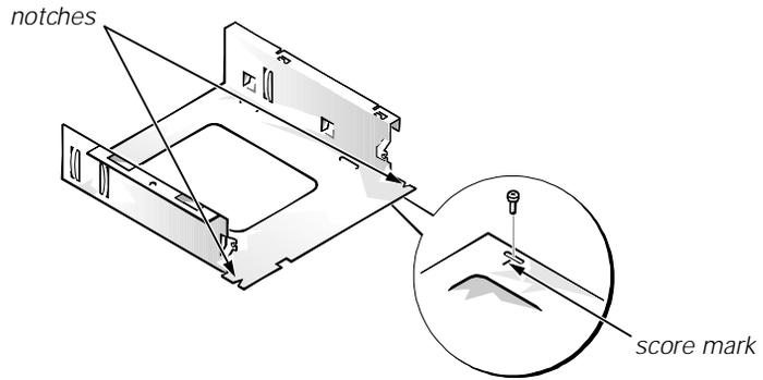
**Figure 7-8. Installing a Drive in the 5.25-Inch Drive Bracket**
