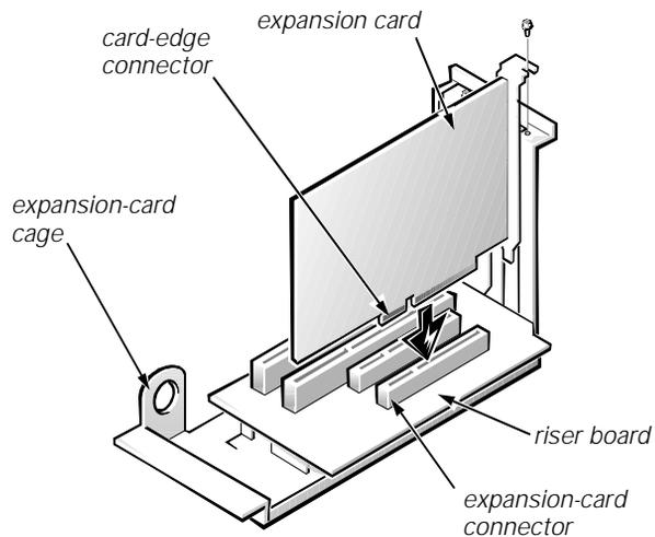
**Figure 6-5. Installing an Expansion Card**
