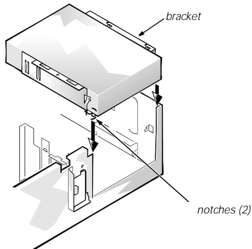
**Figure 7-9. Inserting the Drive Bracket into the Drive Bay**
