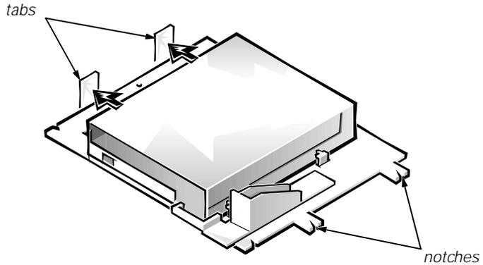
**Figure 7-6. Removing the 3.5-Inch Diskette Drive/Bracket Assembly**
