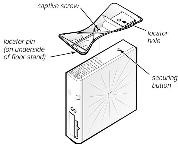
**Figure 1-3. Attaching the Optional Stand for Vertical Orientation**
