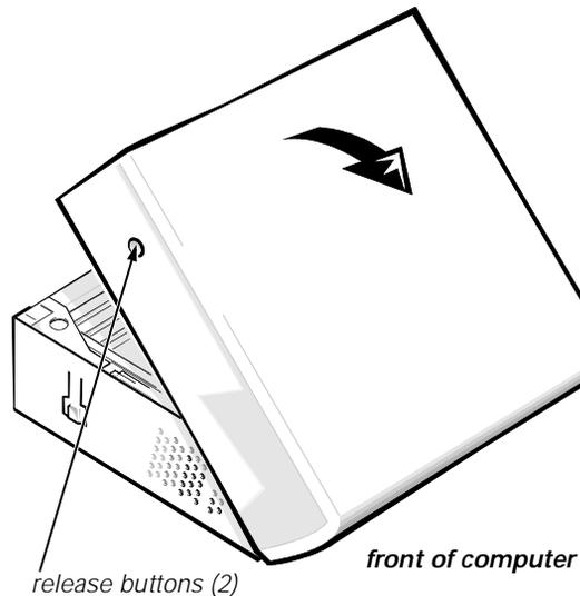
**Figure 5-2. Removing the Computer Cover**
