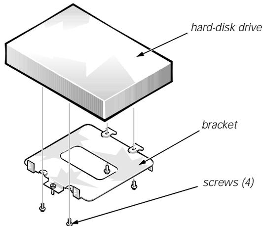
**Figure 7-12. Securing the Hard-Disk Drive to the Bracket**
