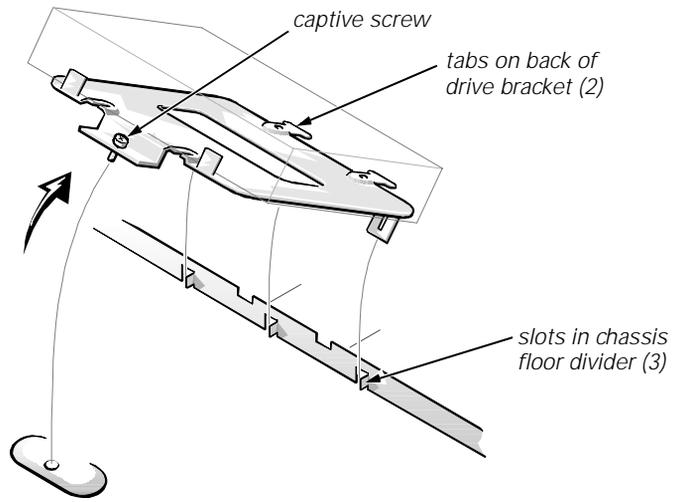
**Figure 7-11. Removing the Hard-Disk Drive Bracket**
