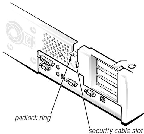
**Figure 1-2. Security Cable Slot and Padlock Ring**
