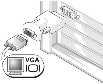
Use the VGA adapter when you have a single-monitor graphics card and you want to connect your computer to a VGA monitor.
