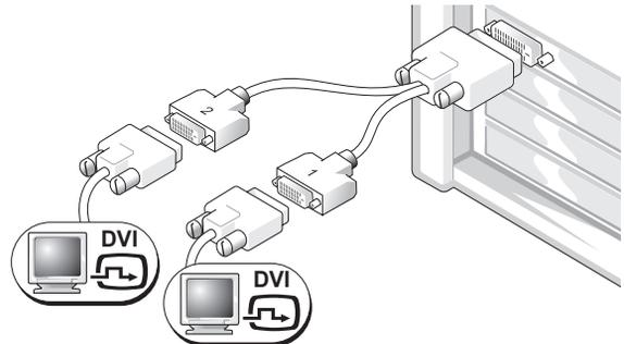
Use the appropriate Y cable when your graphics card has a single connector and you want to connect your computer to one or two DVI monitors.
