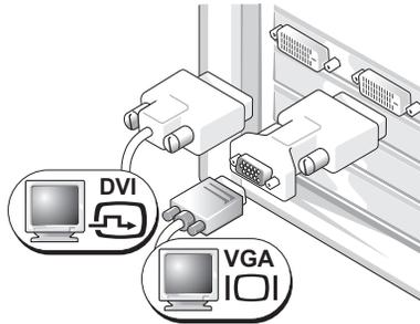
Use the VGA adapter to connect a VGA monitor to one of the DVI connectors on your computer
