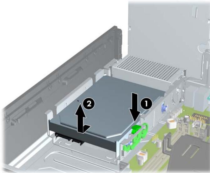
11. To install a hard drive, you must transfer the silver and blue isolation mounting guide screws from the old hard drive to the new hard drive.
