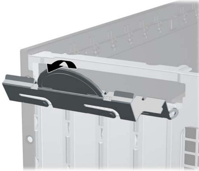
9. Before installing an expansion card, remove the expansion slot cover or the existing expansion card.
