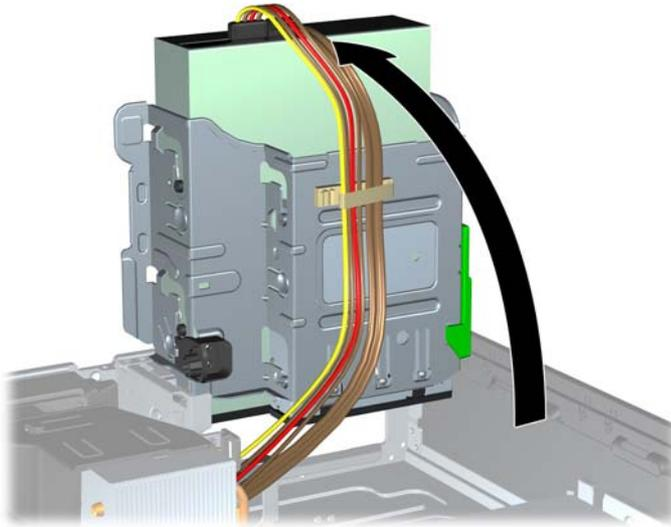
8. Rotate the power supply to its upright position. The hard drive is located beneath the power supply.
