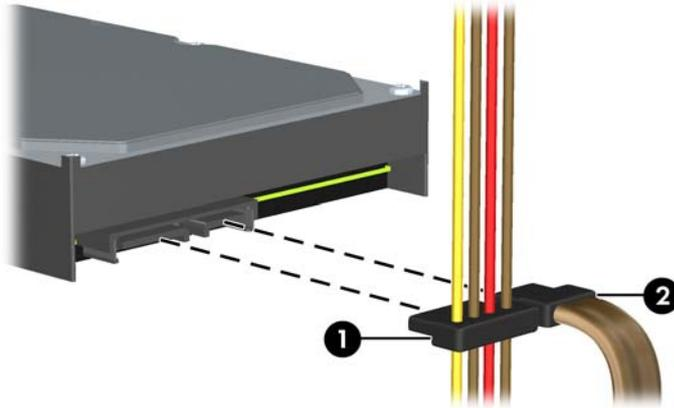
10. Press down on the green release latch next to the hard drive (1). While holding the latch down, slide the drive forward until it stops, then lift the drive up and out of the bay (2).
