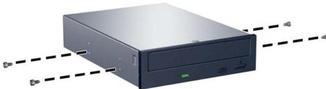
6. Position the guide screws on the drive into the J-slots in the drive bay. Then slide the drive toward the front of the computer until it locks into place.
