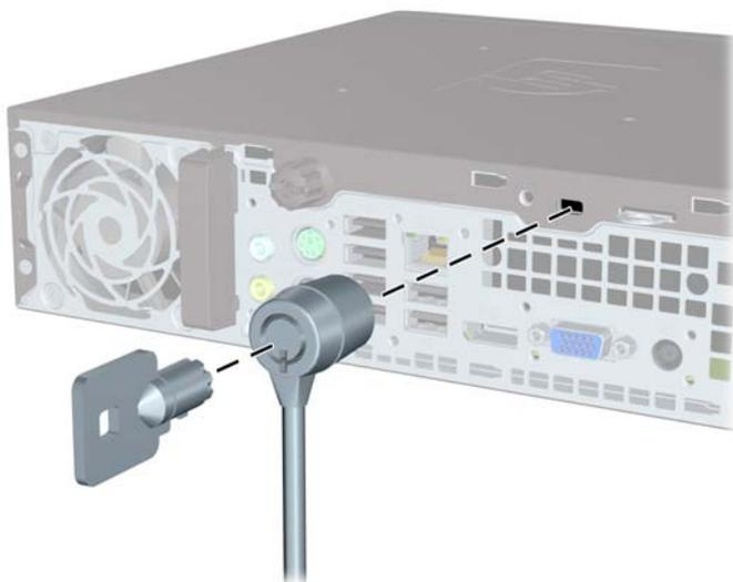
**Figure 7-2** Installing a Cable with a Port Cover Installed
