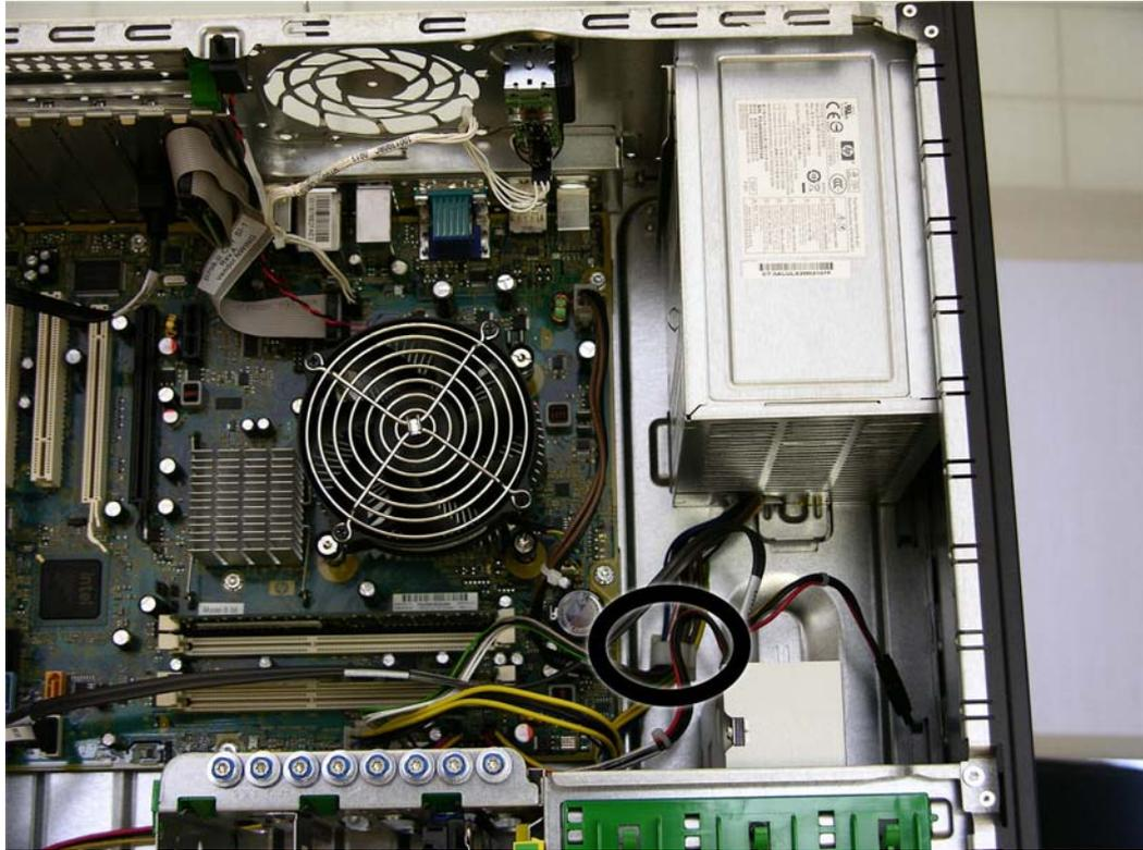
5. Remove the two Torx screws (1) and the two security screws (2) that connect the power supply to the chassis.
