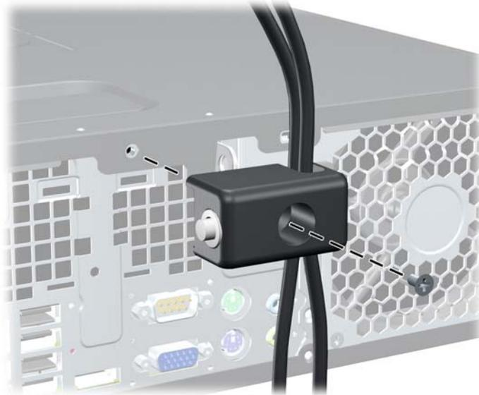
4. Insert the plug end of the security cable into the lock (1) and push the button in (2) to engage the lock. Use the key provided to disengage the lock.
