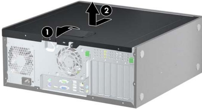
To install the access panel, reverse the removal procedure.
