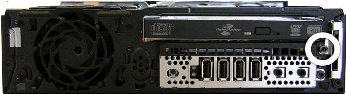
6. Pull the reader away from the front of the chassis while threading the cable through the slot in the front of the chassis.
