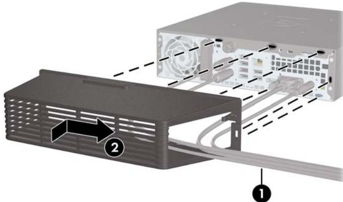
**NOTE:** For security purposes, you can install an optional cable lock to the chassis that locks the port cover and secures the computer. See [Installing a Security Lock on page 144](#).
