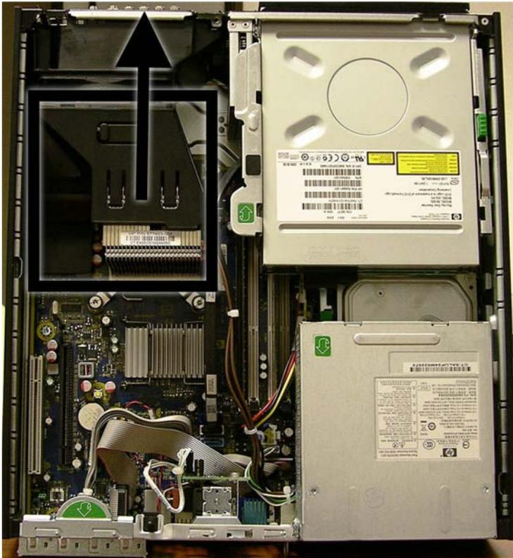
To install the baffle, reverse the removal procedure.
