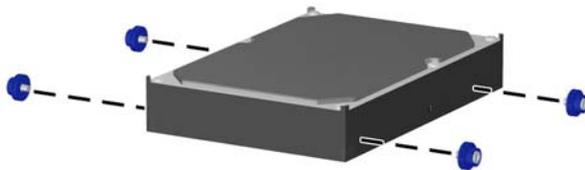
9. Align the guide screws with the slots on the chassis drive cage, press the hard drive down into the bay, then slide it back until it stops and locks in place.
