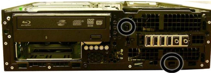
7. Pull the assembly toward the rear of the unit, and then lift it out of the chassis.
