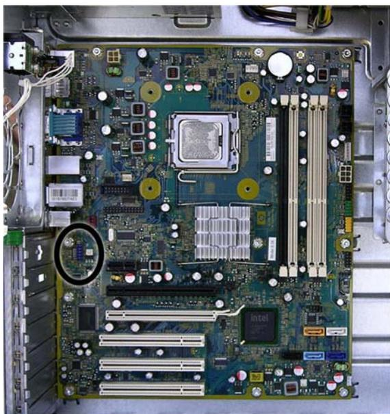
5. Remove the screw that secures the assembly to the front of the chassis **(1)**.
