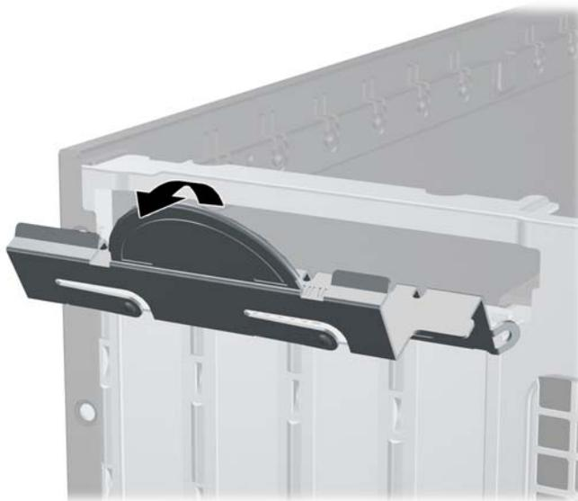
5. Before installing an expansion card, remove the expansion slot cover or the existing expansion card.
