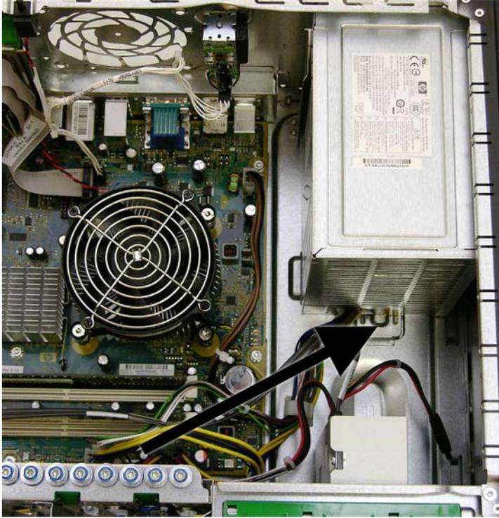
7. Slide the power supply toward the front of the computer, rotate toward the fan so the power supply clears the lip on the top of the chassis, and then lift the power supply out of the chassis.
