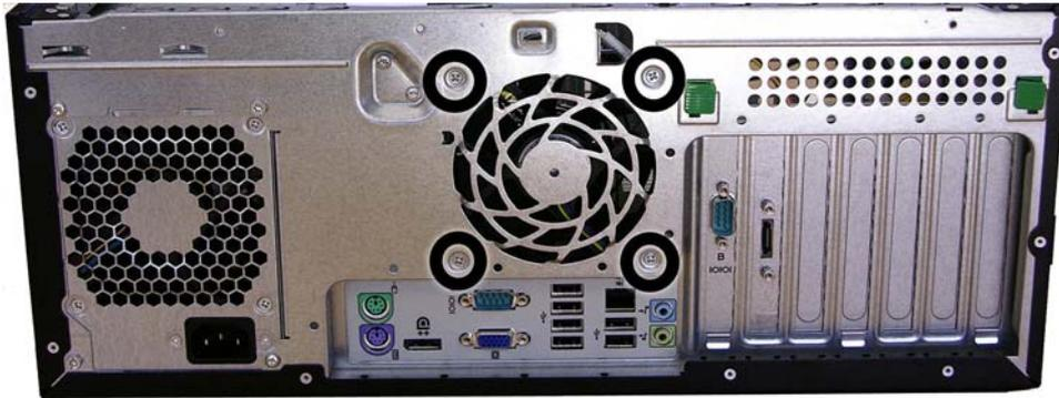
To install the fan, reverse the removal procedure. Be sure to orient the air flow out of the unit.
