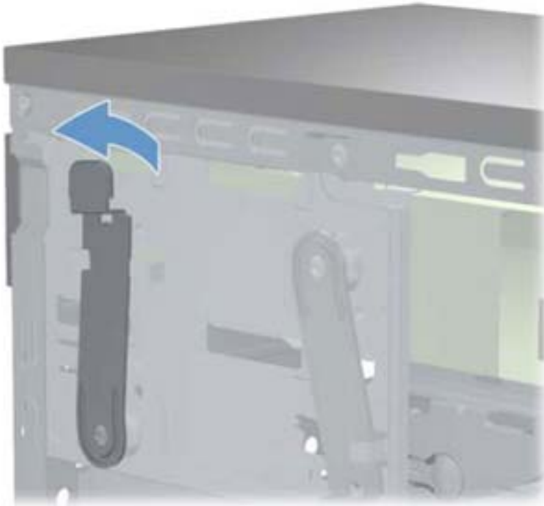
Figure 7-24 Pushing the optical drive
