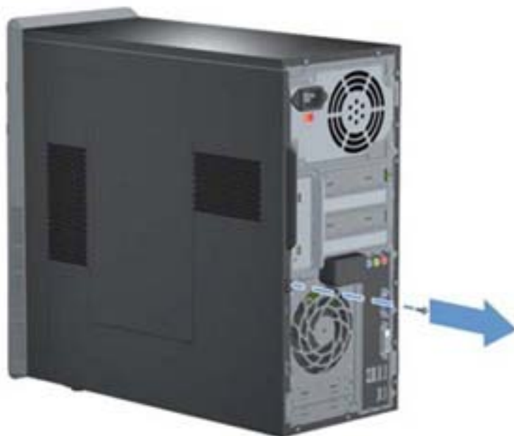
Figure 7-1 Removing the access panel screw
