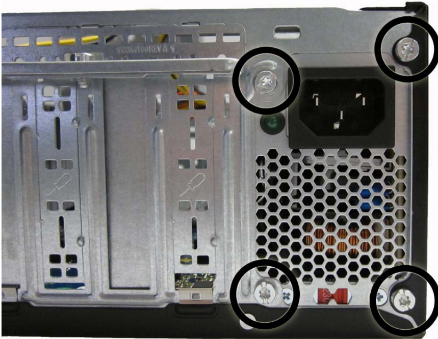
Figure 8-36 Removing the power supply screws
