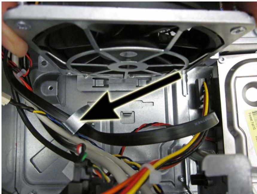
Figure 8-26 Removing the cables from the clip
