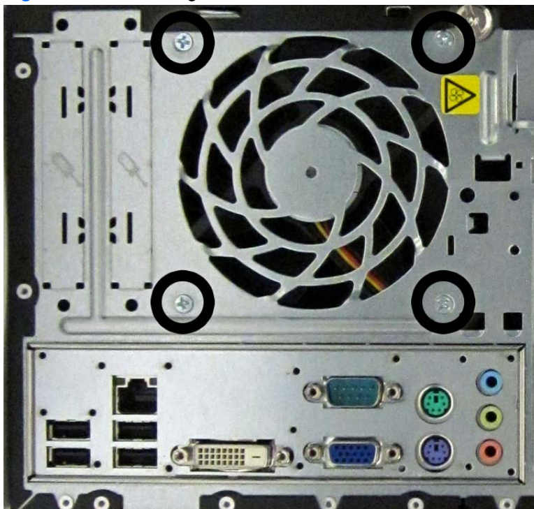
Figure 7-41 Removing the fan screws
