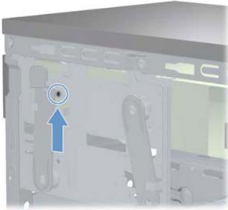
Figure 7-28 Optical drive alignment hole
