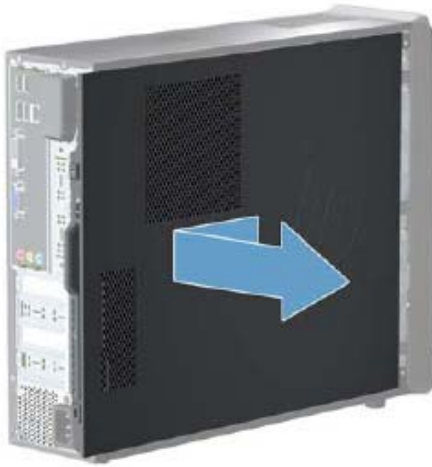
Figure 8-2 Removing the access panel
