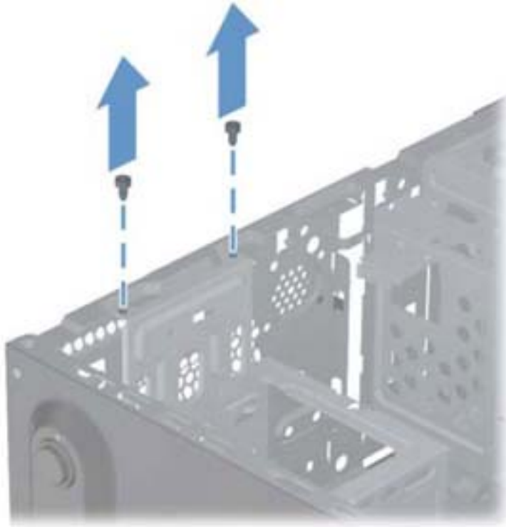
Figure 7-30 Removing the hard drive cage screws
