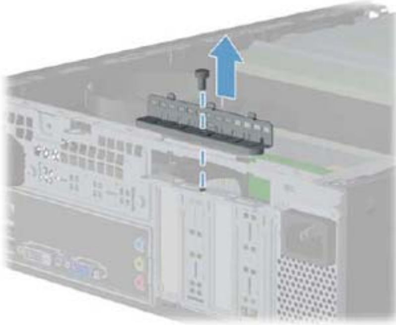
Figure 8-10 Opening the expansion slot bracket
