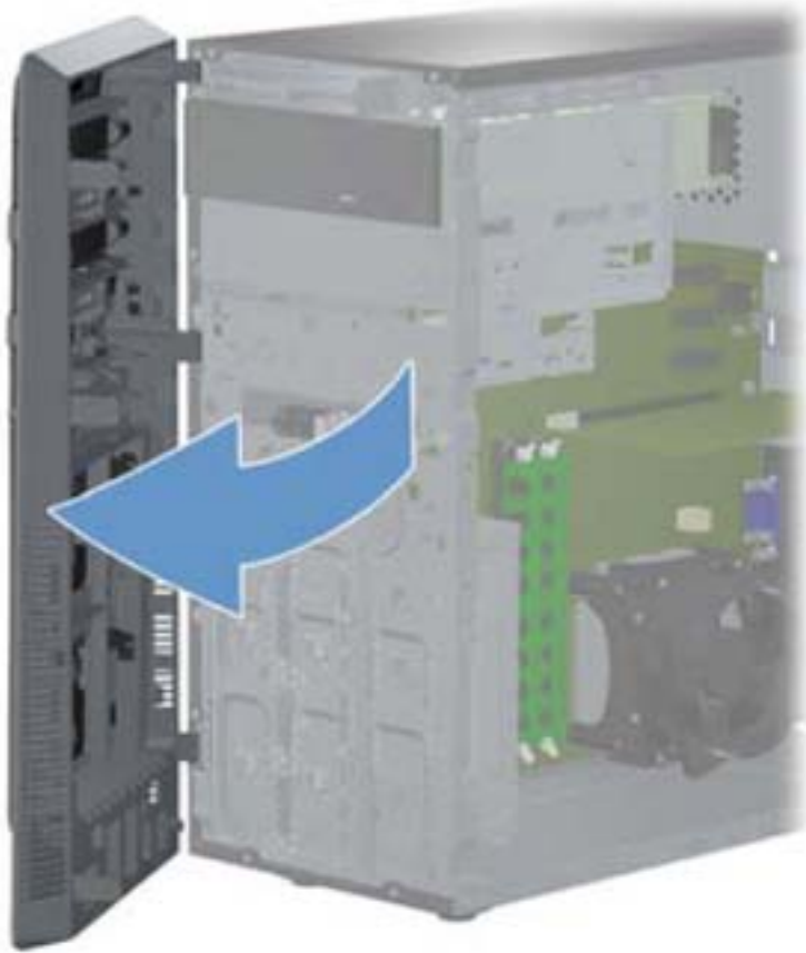
Figure 7-4 Removing the Front Bezel
