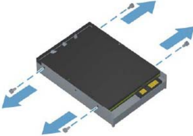
Figure 8-22 Removing the hard drive guide screws
