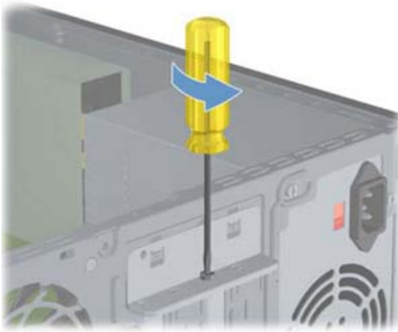
Figure 7-14 Opening the slot cover lock
