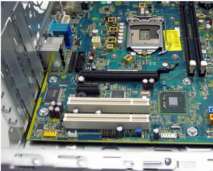
Figure 7-17 Expansion slot locations (HP Pro 3330/3380 shown)
