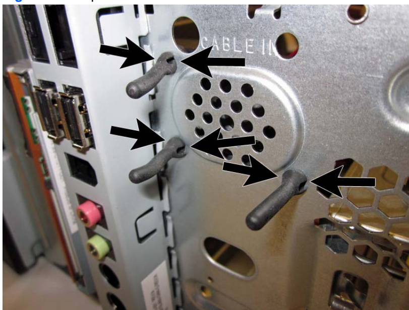
Figure 7-43 Speaker rubber rivets
