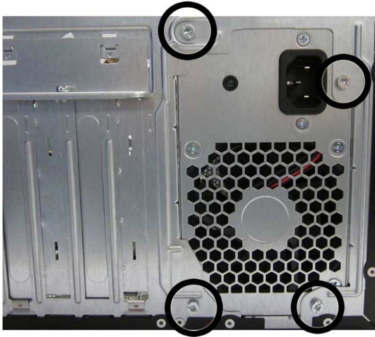
Figure 7-48 Power supply screws
