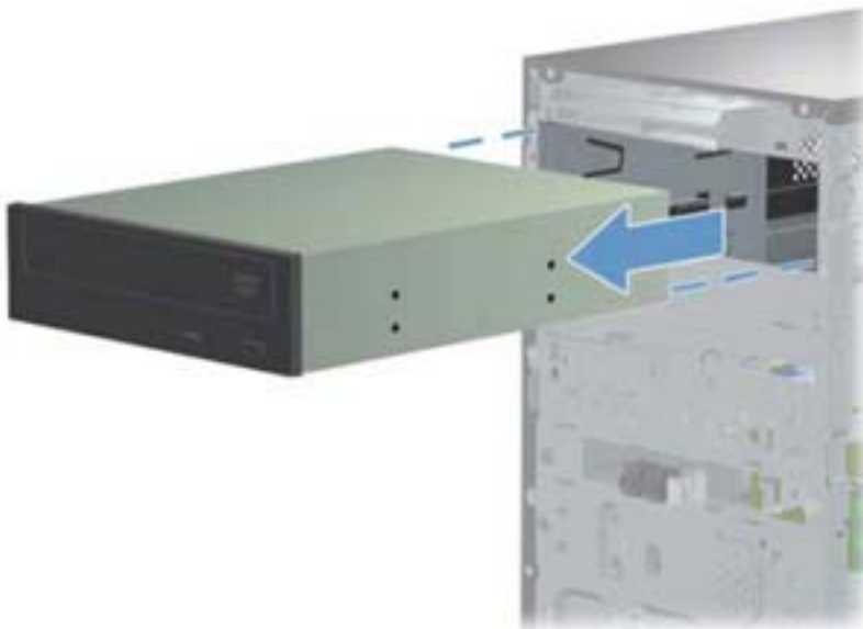
Figure 7-27 Removing the drive
