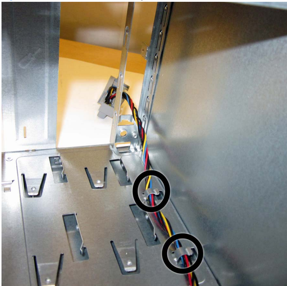
Figure 7-39 Power switch cable routing
