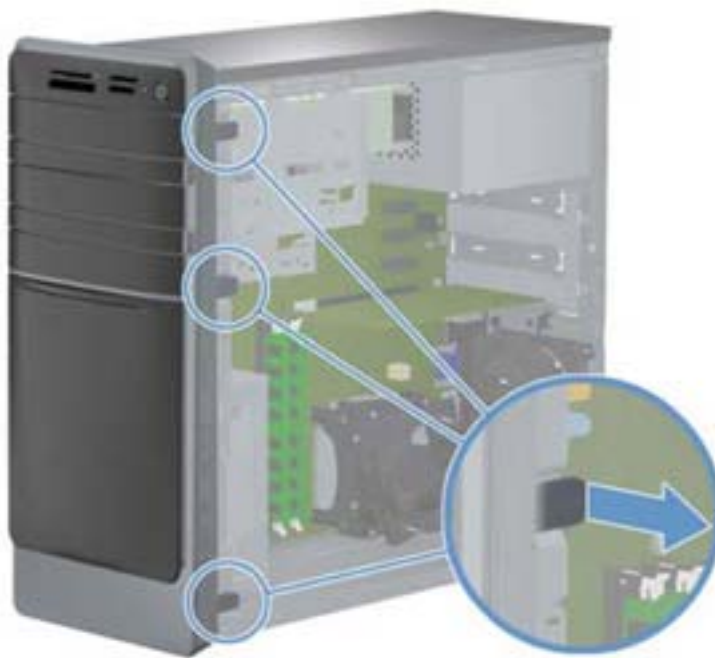
Figure 7-3 Removing the Front Bezel
