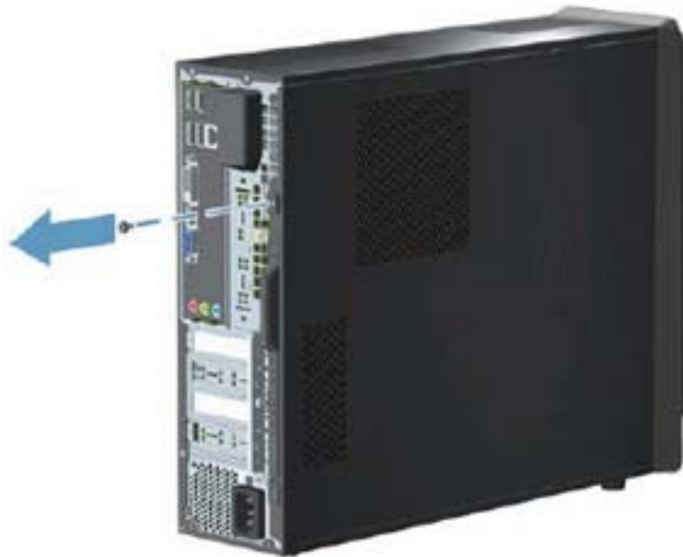
Figure 8-1 Removing the access panel screw
