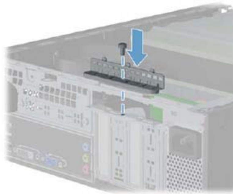
Figure 8-13 Replacing the expansion slot bracket
