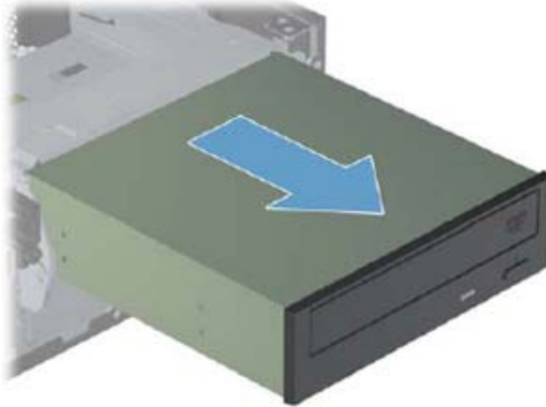
Figure 8-17 Removing the optical drive
