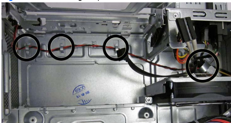
Figure 8-23 Removing the power switch cable
