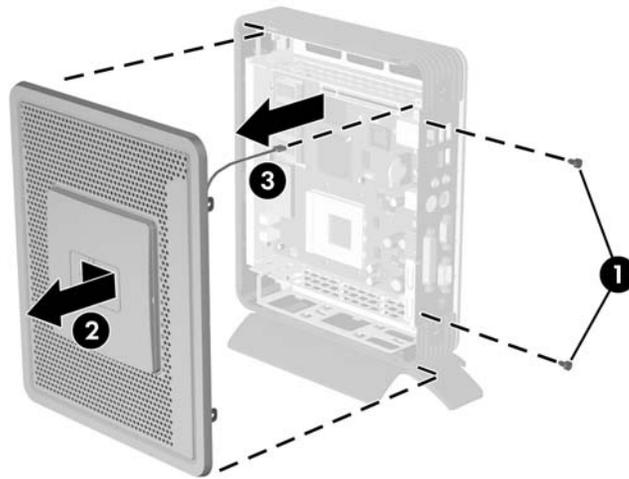
*Removing the chassis cover and disconnecting the speaker*
