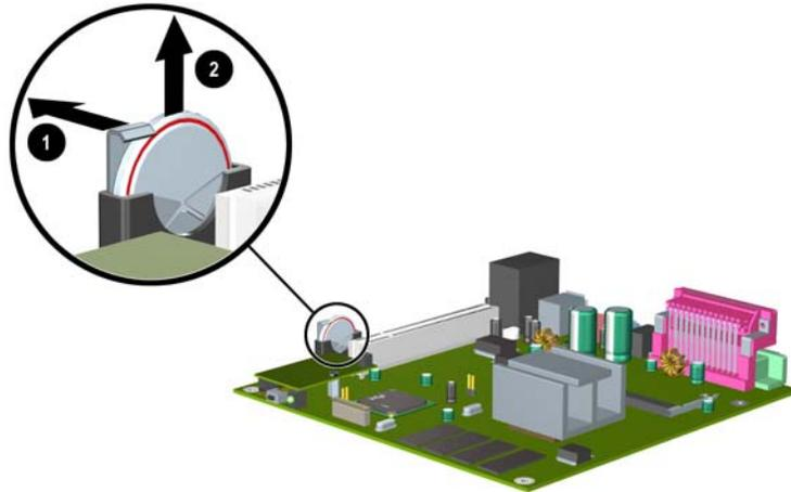
*Removing and Replacing the CMOS Battery*
