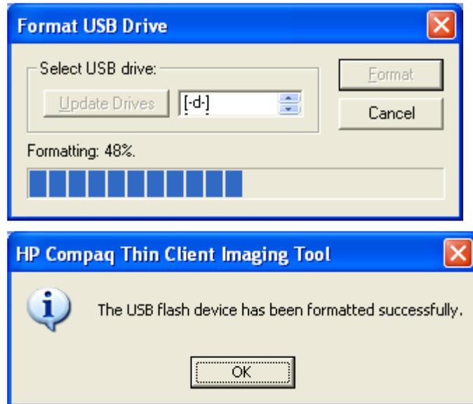
Connect the bootable USB flash device to the thin client. **Only one bootable USB device may be attached to the thin client during this process.**
