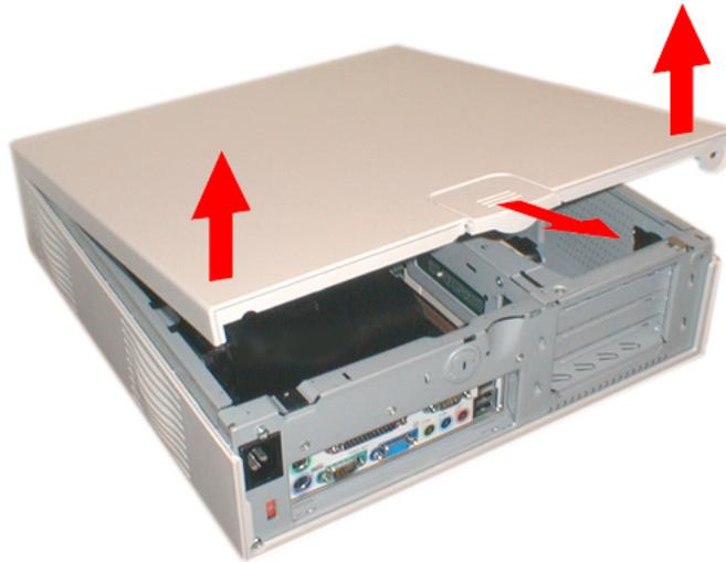
Shows how to remove the front panel
