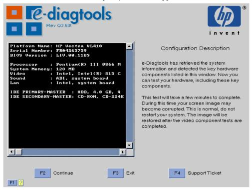
4 Press <**F2**> and the basic system testing starts.
