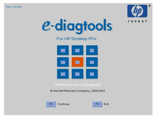
Press <F2> to continue running e-Diagtools hardware diagnostics. You will enter the first phase, hardware detection, described in chapter 4, "e-Diagtools Hardware Detection".
