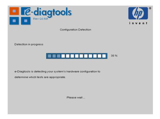
Hardware detection finds and lists the computer's major hardware components. It also determines which tests are appropriate for your computer. For example, if your computer has an IDE or SCSI hard disk drive, it will be checked as part of the basic system test.
