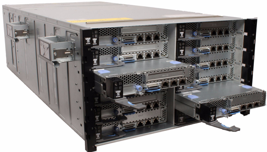
Figure 1 The NeXtScale n1200 Enclosure with twelve compute nodes installed
