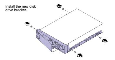
4. Repeat steps 1 to 3 as many times as is necessary to install the new disk drive brackets onto your 1-inch high disk drives.
