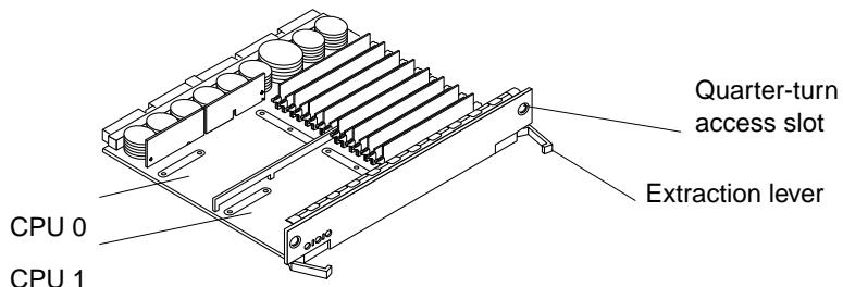
3. Pull both extraction levers outward simultaneously, then pull the board out of the card cage and place it component-side up on the padded ESD mat.
