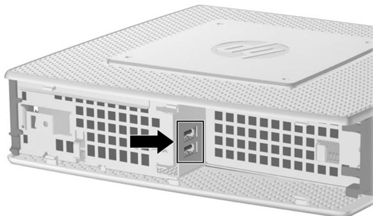
If you install a USB mouse and a USB keyboard in the secure USB compartment, route the cables around and through the clips, then out the secure cable routing slot, as shown in the following illustration.
