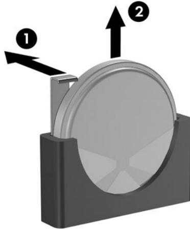
3. To insert the new battery, align the replacement battery with the positive side toward the rear of the unit. Slide one edge of the battery into the slot and push down until the guard snaps over the edge of the battery (2).
