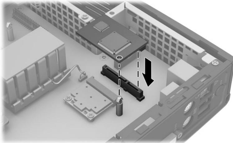
2. Insert the flash memory module into the socket on the system board.
