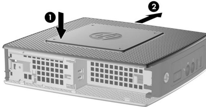
3. Replace the secure compartment cover. For more information, see [Replacing the Secure USB Compartment Cover on page 11](#).
