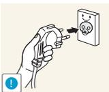
Ensure you connect the power cable to a grounded power socket. (type 1 insulated devices only).
