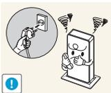
If the product generates a strange noise, a burning smell, or smoke, remove the power cable immediately and contact Samsung Customer Service Center (page 47).
