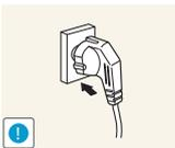
Insert the power cable all the way in so it is not loose.
