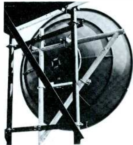
Horizontal Tilt Mount , elevation adjustment -5^{\circ} to +50^{\circ} . Type 19478 for use with four and six foot reflectors Type 31390 for use with eight and ten foot reflectors. Mount to flat surfaces.
