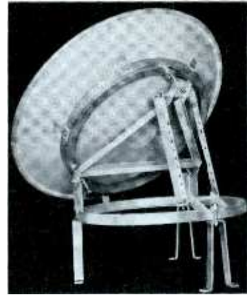
Horizontal Tilt Mount , elevation adjustment -5^{\circ} to +50^{\circ} . Type 19478 for use with four and six foot reflectors Type 31390 for use with eight and ten foot reflectors. Mount to flat surfaces.
